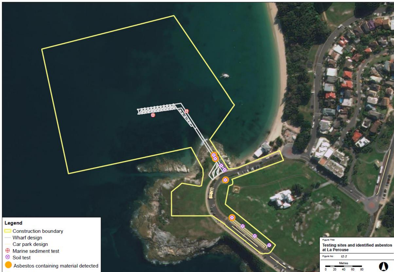
Figure 17-7: Testing sites and identified asbestos containing material (ACM) at La Perouse
