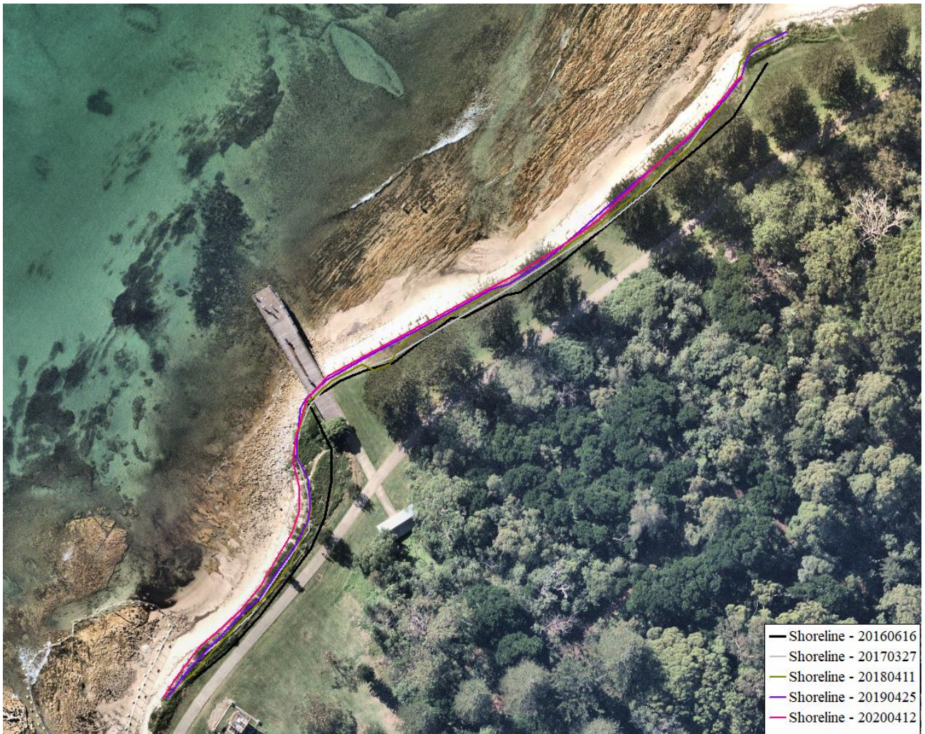
Figure 1-11 Change in the Vegetation Line between June 2016 and April 2020 (image is from 12 April 2020)
