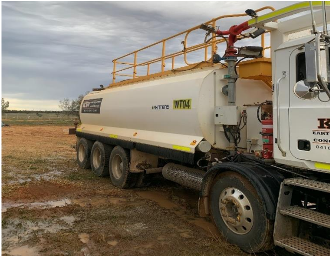
Photo 5: Water cart used for dust suppression and high-pressure cleaning for weed hygiene
