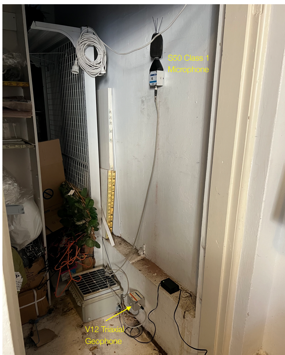
Figure 2: Monitor with V12 Geophone & S50 Microphone (218 Church St)
