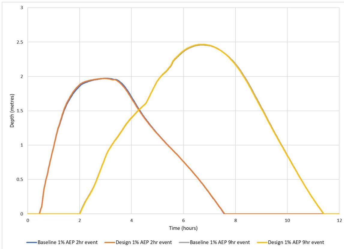
**Figure B-21: Flood level versus time – 1% AEP event, Duck River near Fariola Street, Silverwater**
