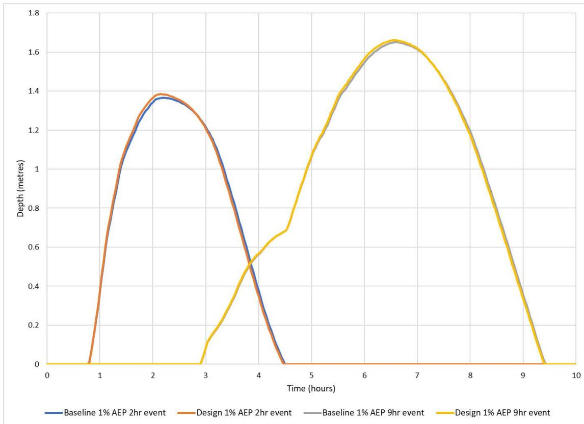
**Figure B-20: Flood level versus time – 1% AEP event, Duck River upstream of M4 Motorway**
