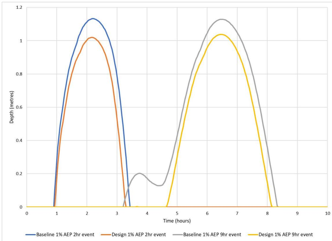
**Figure B-19: Flood level versus time – 1% AEP event, Duck Creek upstream of M4 Motorway**
