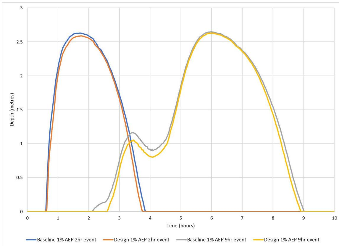
**Figure B-18: Flood level versus time – 1% AEP event, A'Becketts Creek upstream of James Ruse Drive**
