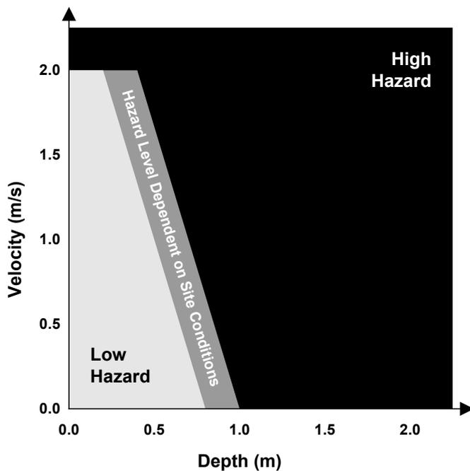
Figure 2-1 *Floodplain Development Manual* flood hazard category diagram (from Figure L2 in *NSW Floodplain Development Manual*)
