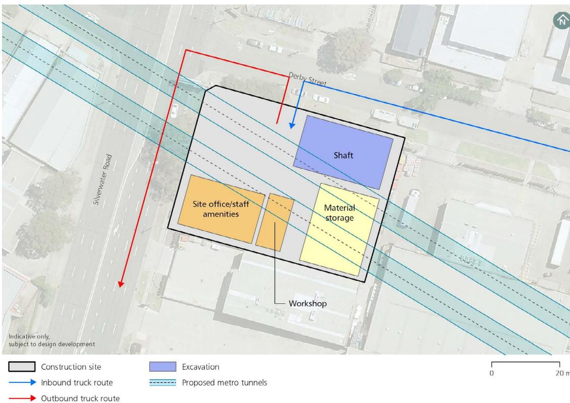
**Figure 2-4: Silverwater services facility construction site**
