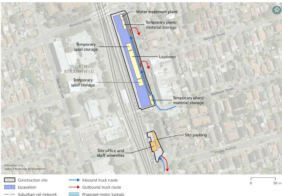
**Figure 2-6: North Strathfield metro station construction site**
