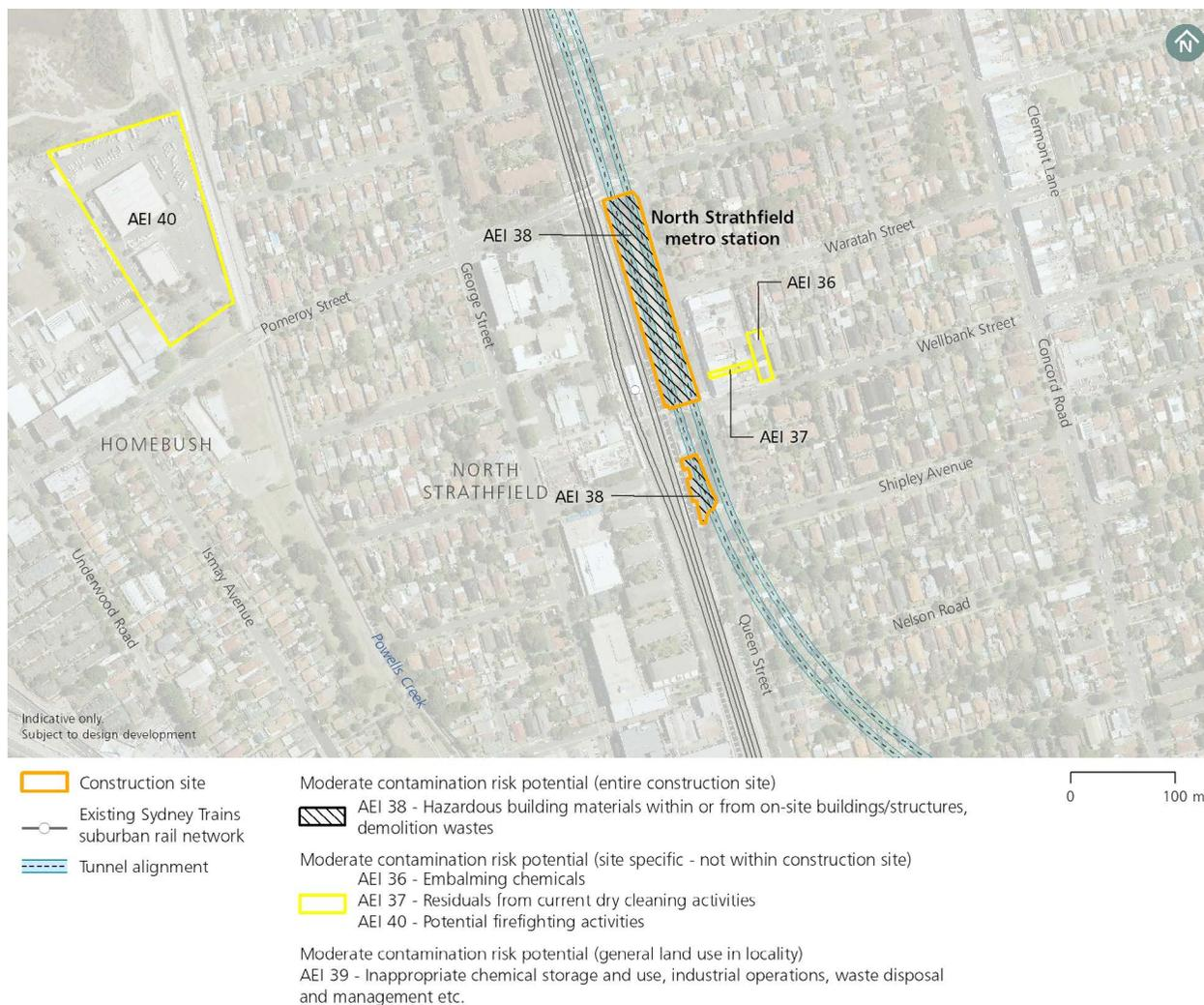
**Figure 4-6: Potential contamination impact – Moderate and above – North Strathfield metro station construction site and alignment**
