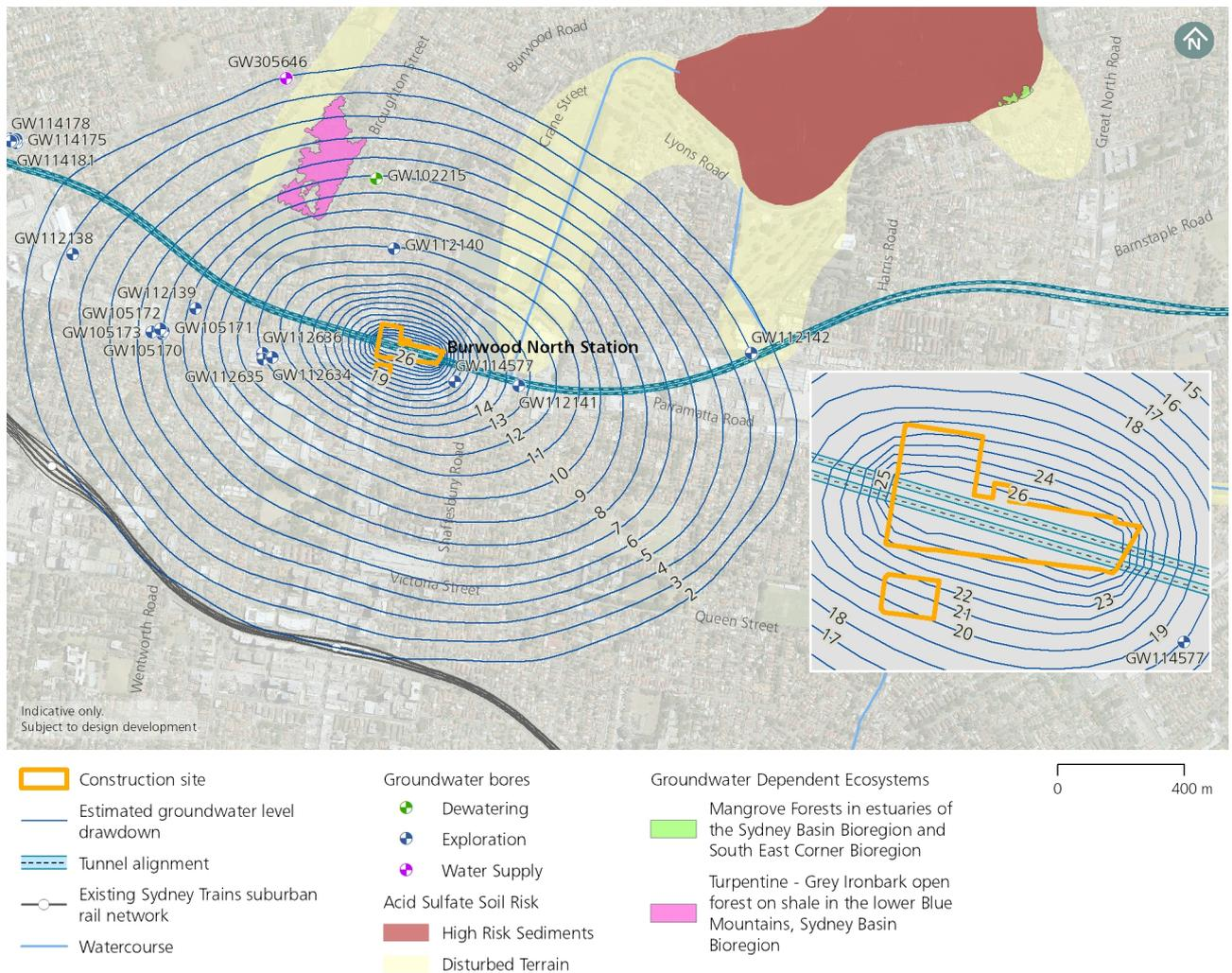
**Figure 5-7: Estimated groundwater level drawdown from the current water level after two years due to Stage 1 excavation at Burwood North Station construction site**
