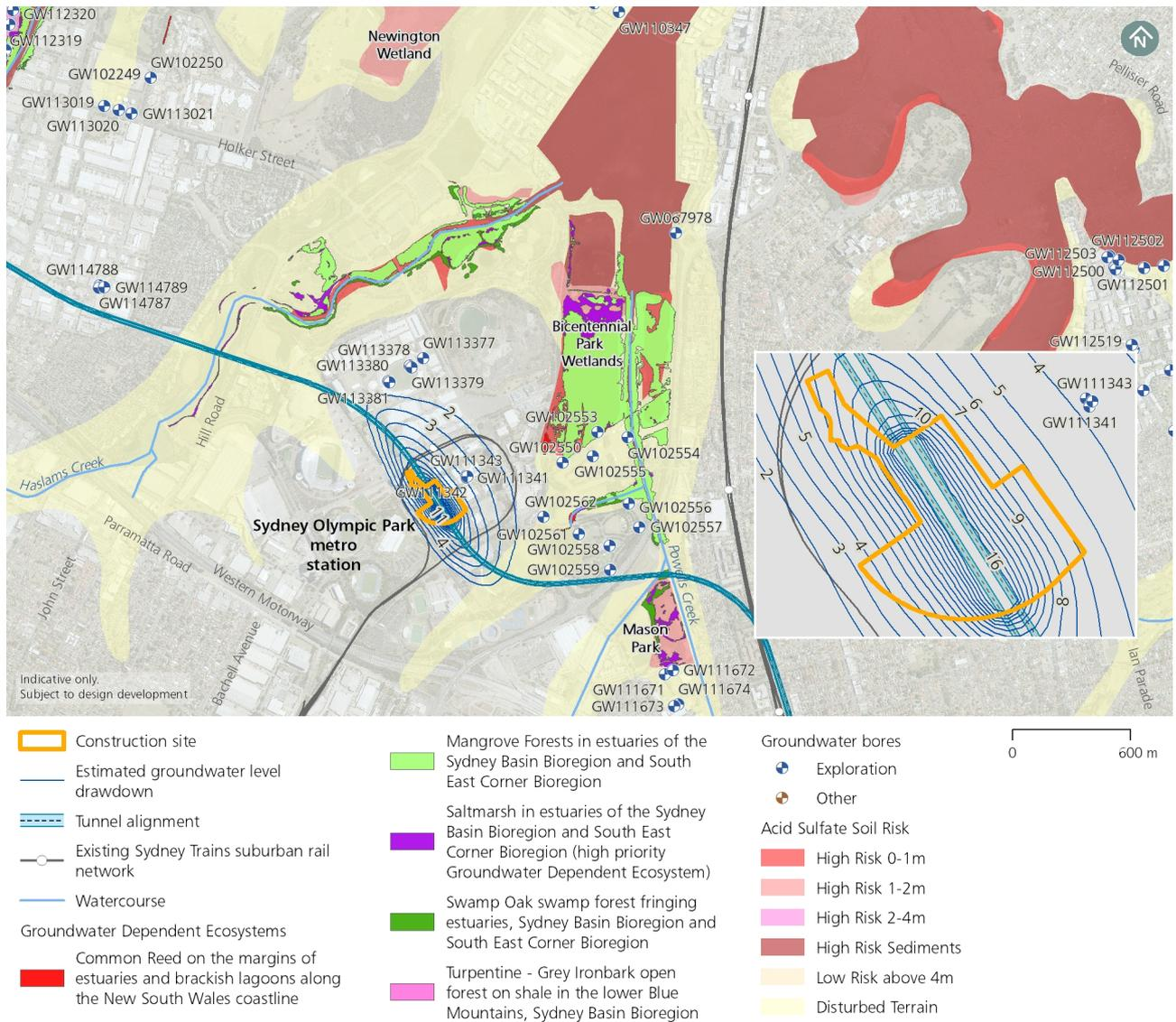
**Figure 5-5: Estimated groundwater level drawdown from the current water level after two years due to Stage 1 excavation at Sydney Olympic Park metro station construction site**
