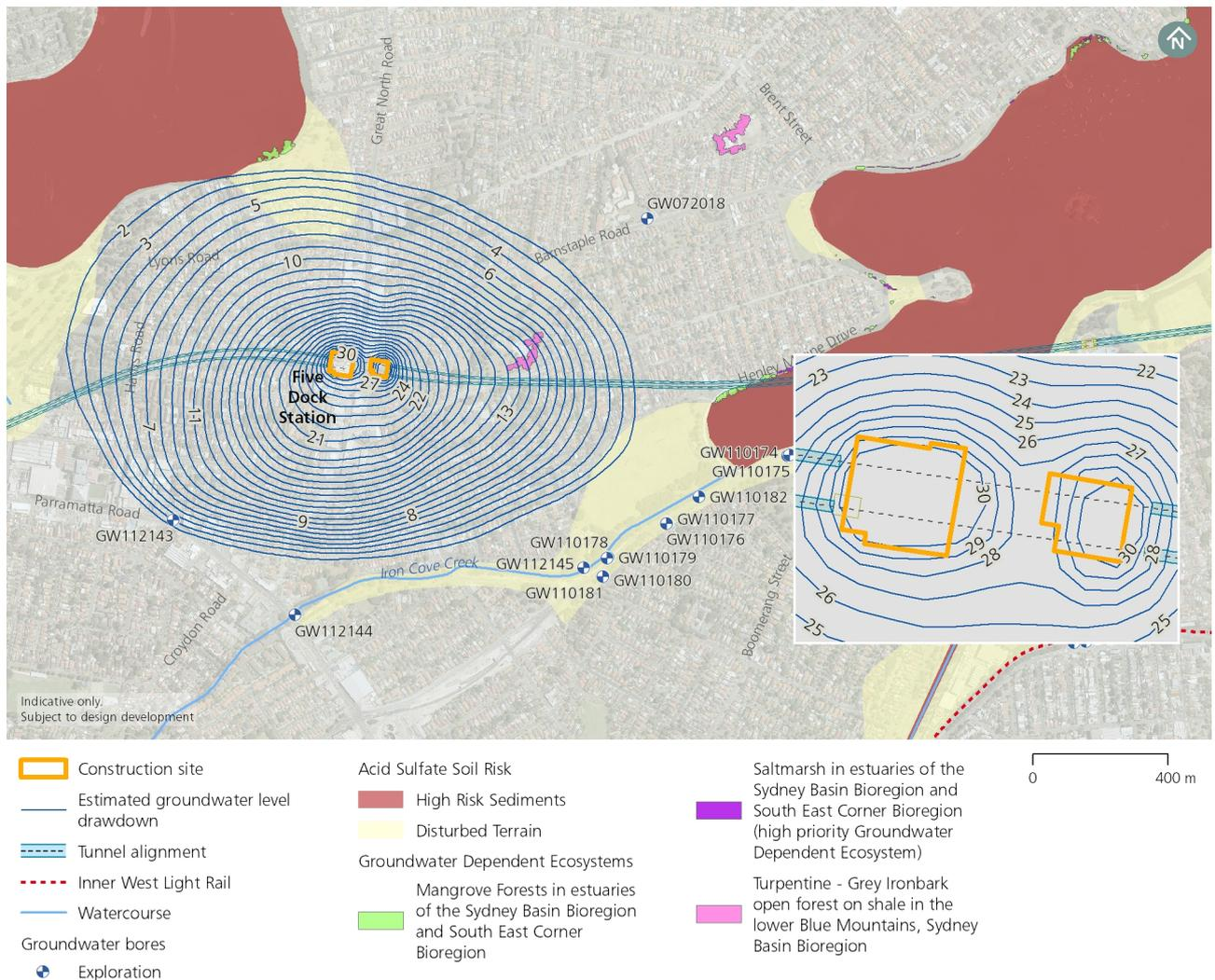
**Figure 5-8: Estimated groundwater level drawdown from the current water level after two years due to Stage 1 excavation at Five Dock Station**
