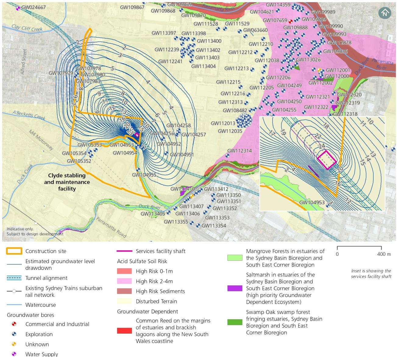
**Figure 5-3: Estimated groundwater level drawdown from the current water level after two years due to Stage 1 excavation at Clyde stabling and maintenance facility construction site**
