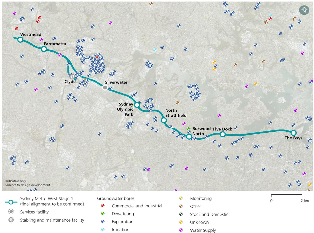
**Figure 4-3: WaterNSW-registered groundwater bores along the Stage 1 alignment**
