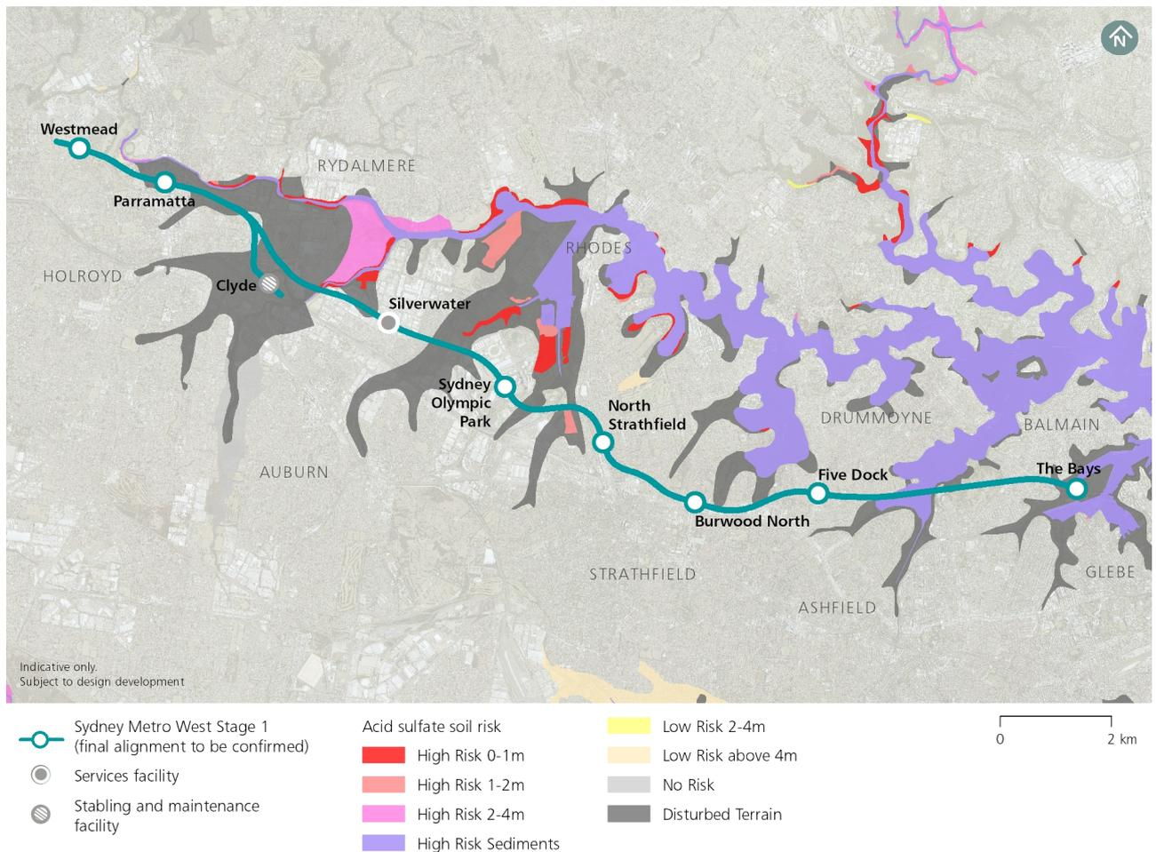
**Figure 4-2: Acid sulfate soils risk along the Stage 1 alignment**
