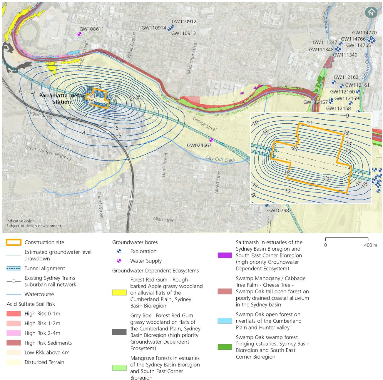
**Figure 5-2: Estimated groundwater level drawdown from the current water level after two years due to Stage 1 excavation at Parramatta metro station construction site**
