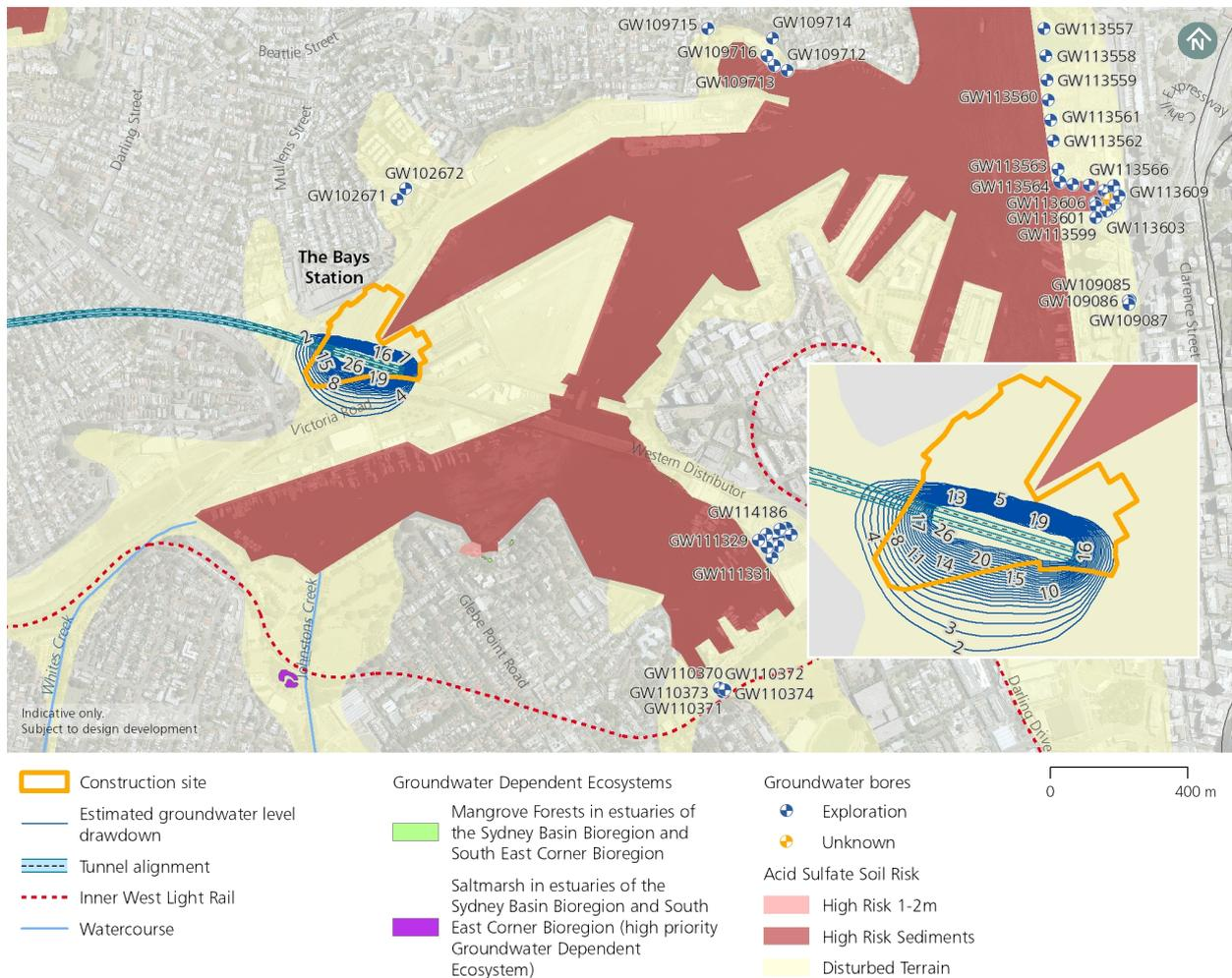
**Figure 5-9: Estimated groundwater level drawdown from the current water level after two years due to Stage 1 excavation at The Bays Station construction site**
