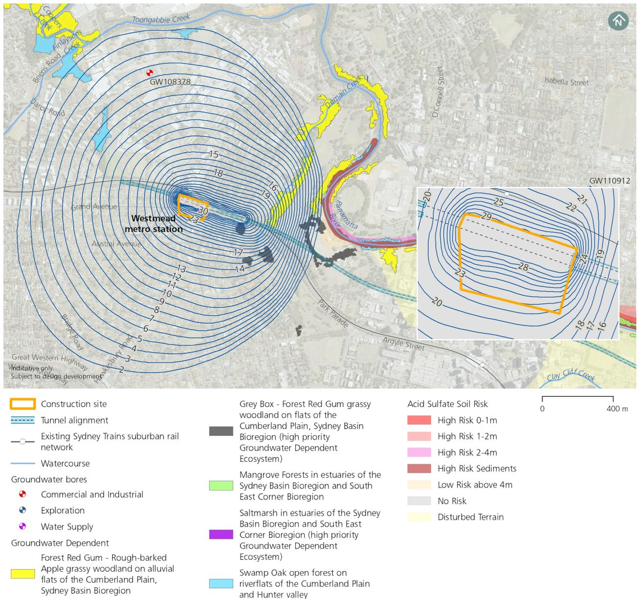
**Figure 5-1: Estimated groundwater level drawdown from the current water level after two years due to Stage 1 excavation – Westmead metro station construction site**
