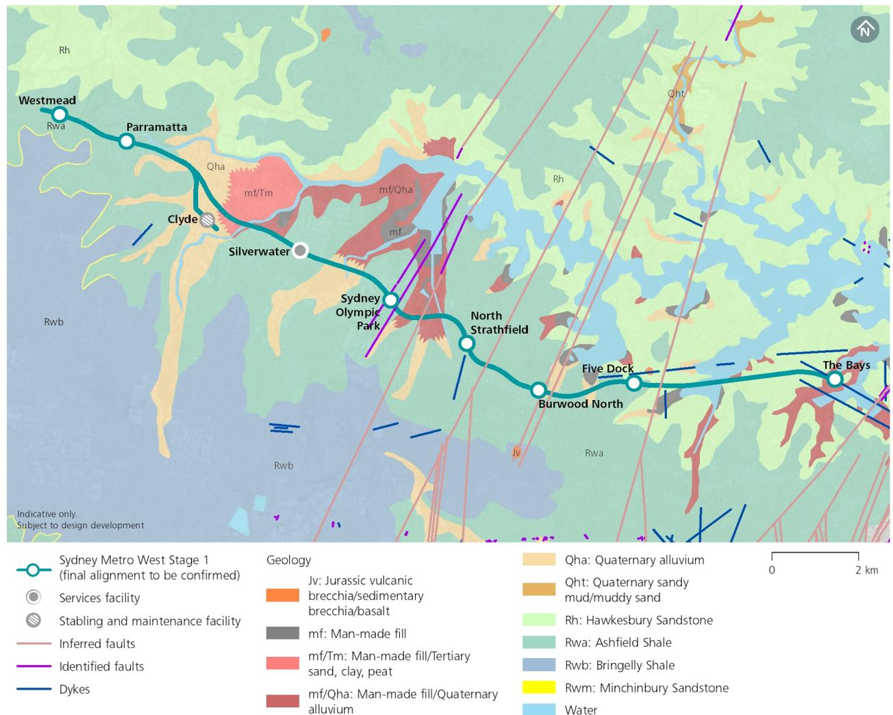
**Figure 4-1: Geology along Stage 1 alignment**
