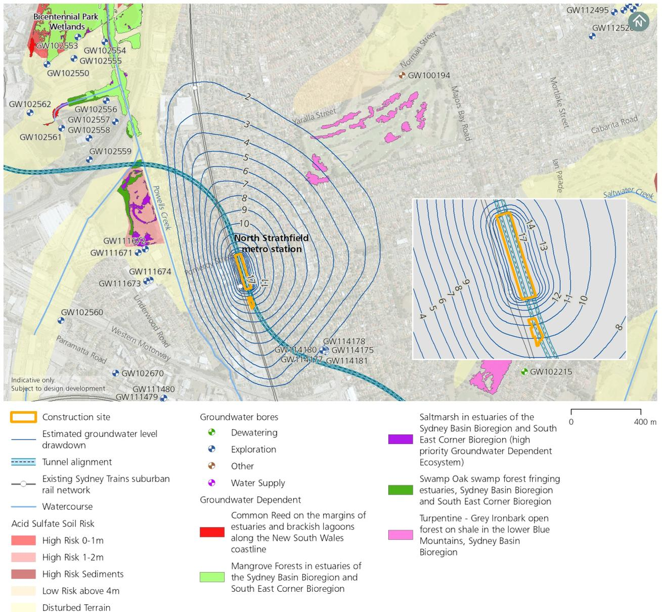
**Figure 5-6: Estimated groundwater level drawdown from the current water level after two years due to Stage 1 excavation at North Strathfield metro station construction site**
