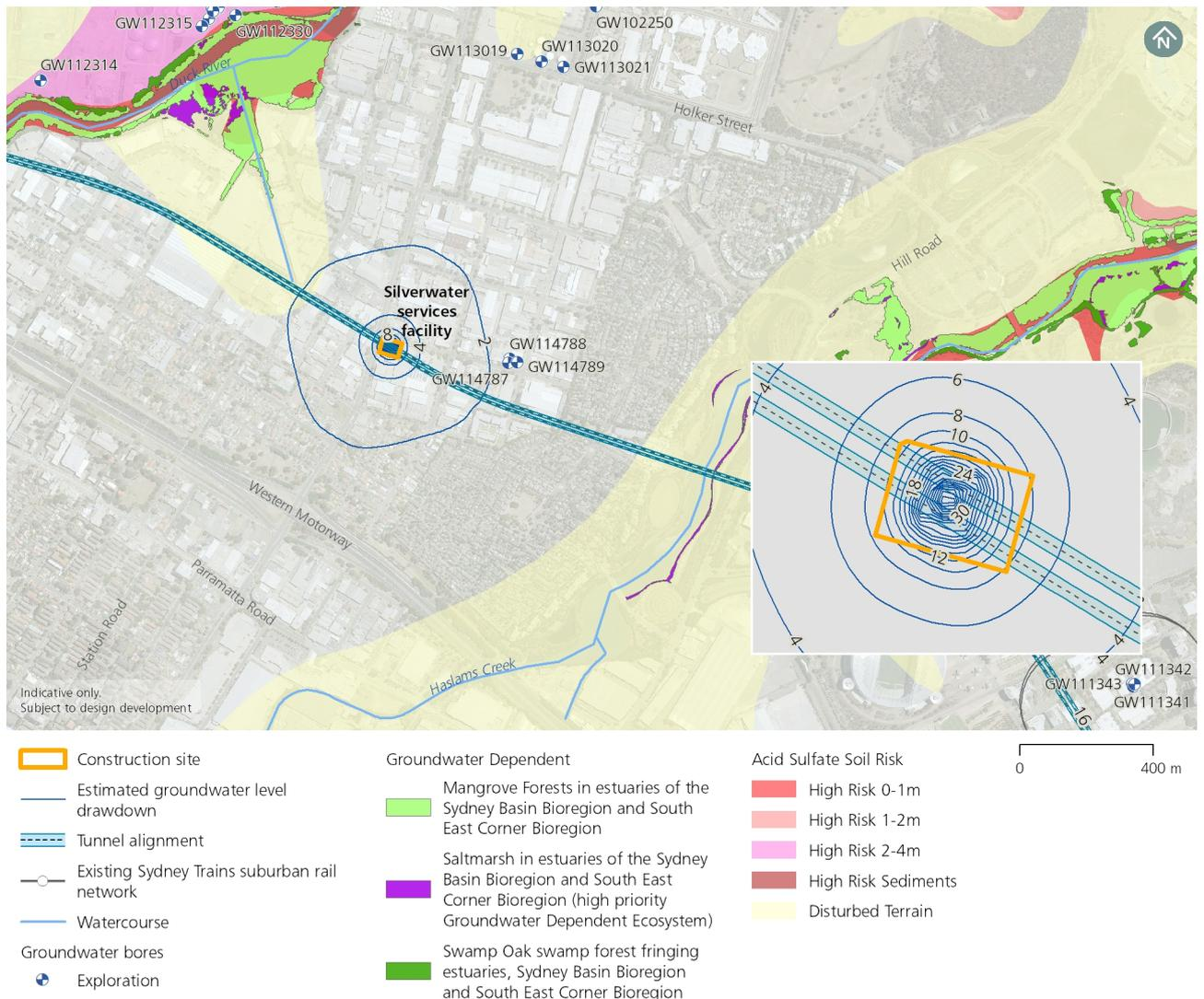
**Figure 5-4: Estimated groundwater level drawdown from the current water level after two years due to Stage 1 excavation at Silverwater services facility construction site**
