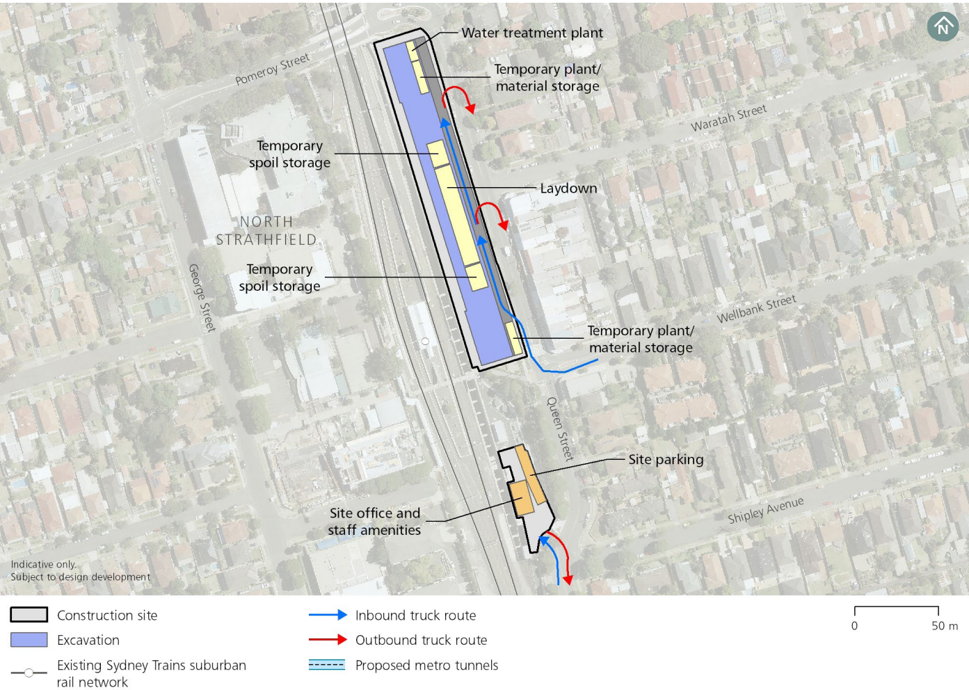
FIGURE 10-3: NORTH STRATHFIELD METRO STATION CONSTRUCTION SITE LAYOUT
