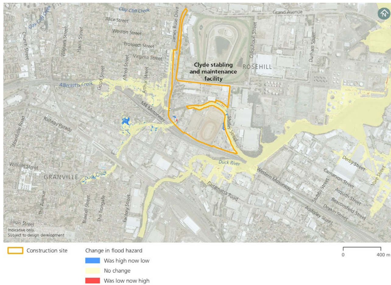
Figure 21-1: Potential change in flood hazard at the Clyde stabling and maintenance facility construction site – five per cent AEP event
