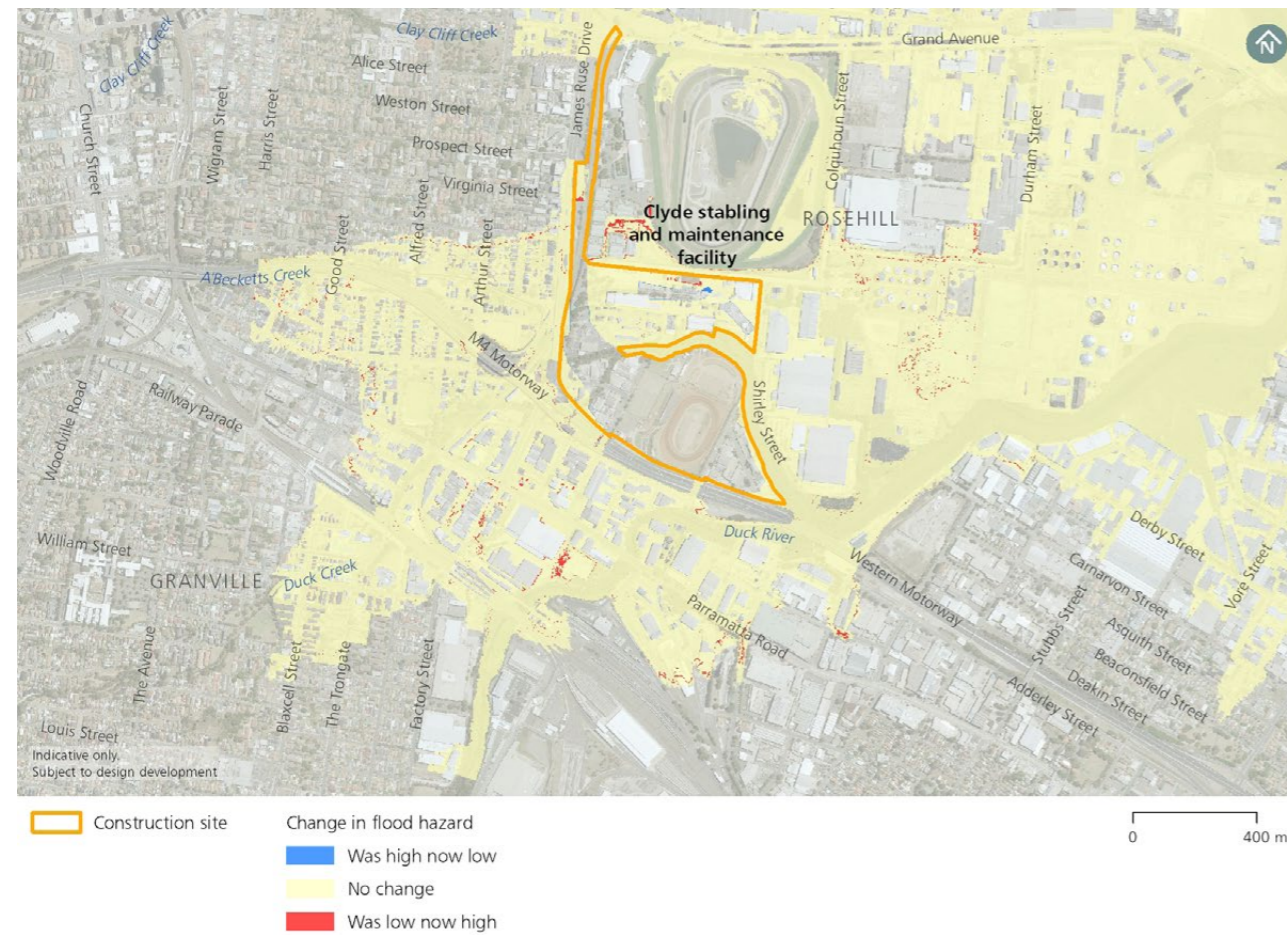
Figure 21-3: Potential change in flood hazard at the Clyde stabling and maintenance facility construction site – PMF event
