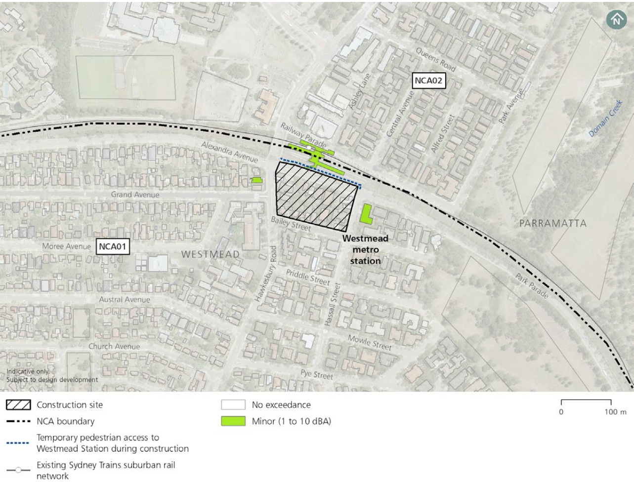
Figure 11-3: Ground-borne noise impacts (daytime construction hours) – Westmead metro station construction site
