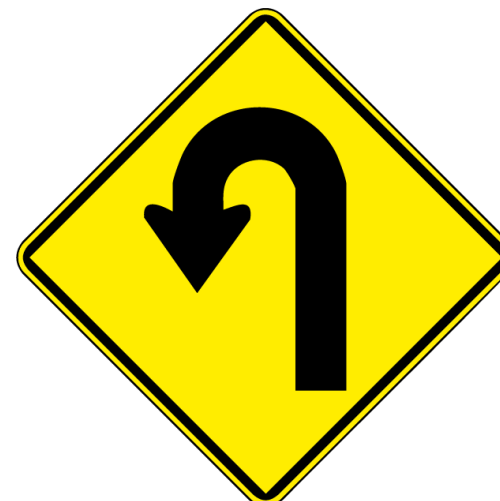
● Warning Signage (Directive)- Hairpin Bend
