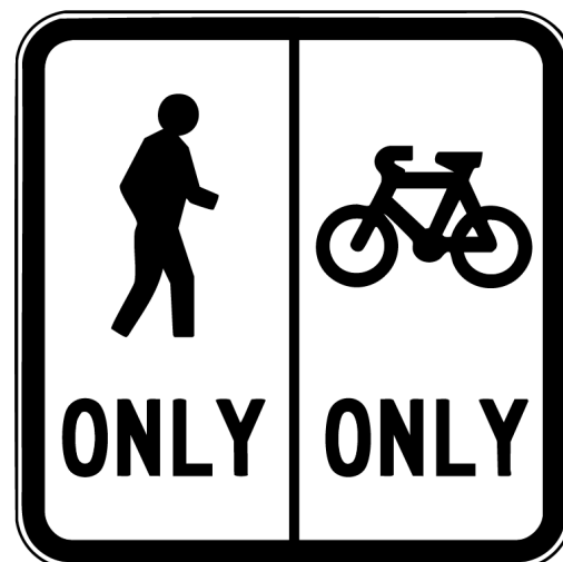
● Regulatory Signage - Separated Path (R8-3(L and R))
