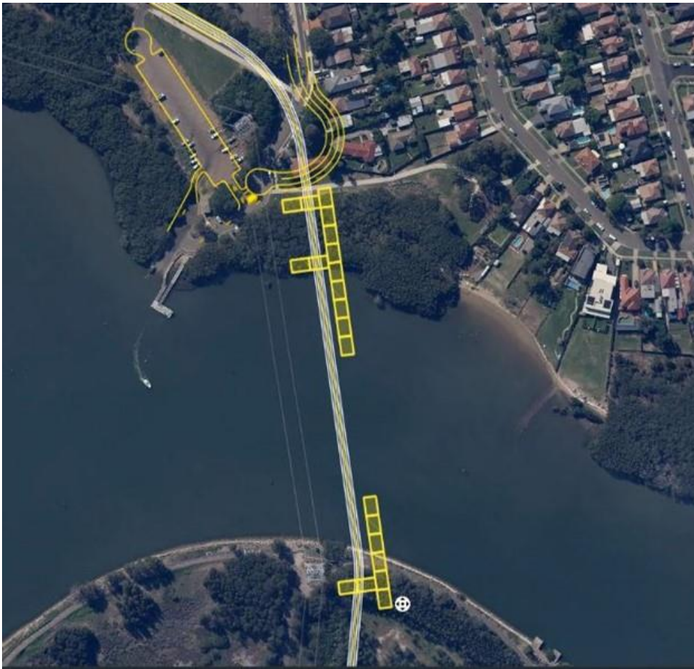
Figure 4.2 Conceptual arrangement of temporary working platforms between Melrose Park and Wentworth Point
