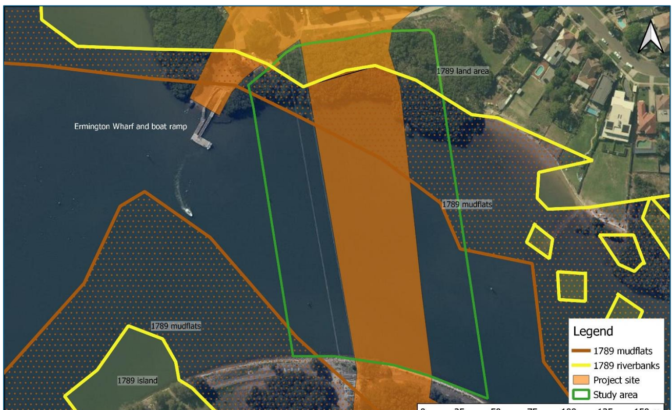
Figure 5-1: The project site and study area overlaid on current aerial map with mudflats and riverbanks derived from a 1789 map. Original riverbank (yellow). Original extent of mud flats (brown). (Source: SLNSW 'Flats at the head of Port Jackson & channel up to Rose Hill' by-W Bradley)
