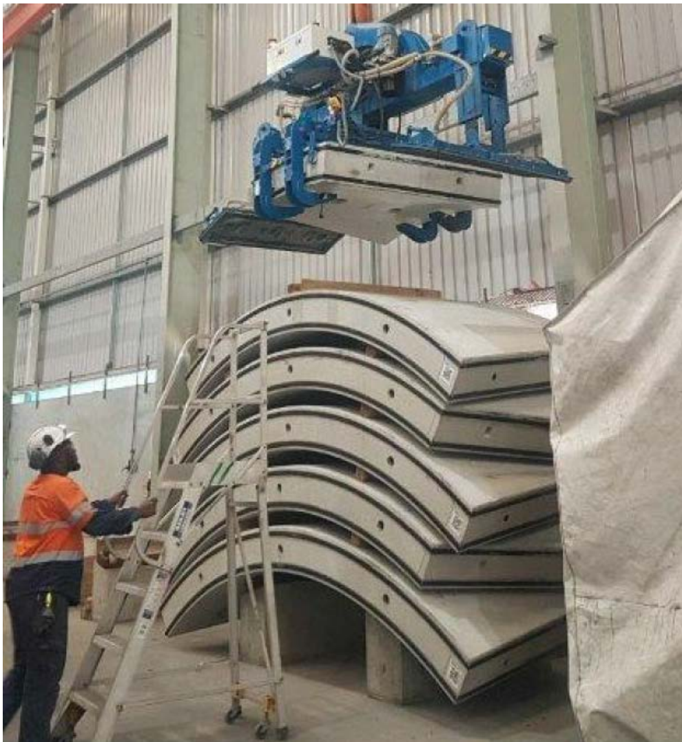
Figure 5 | Finished Concrete Segments
