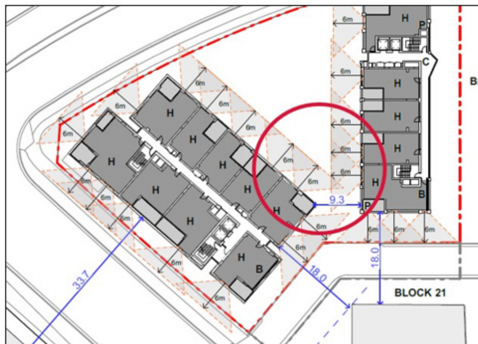
Figure 1 Typical floor plan overlay with red circle highlighting areas where interface conditions of windows and balconies should be reconsidered
