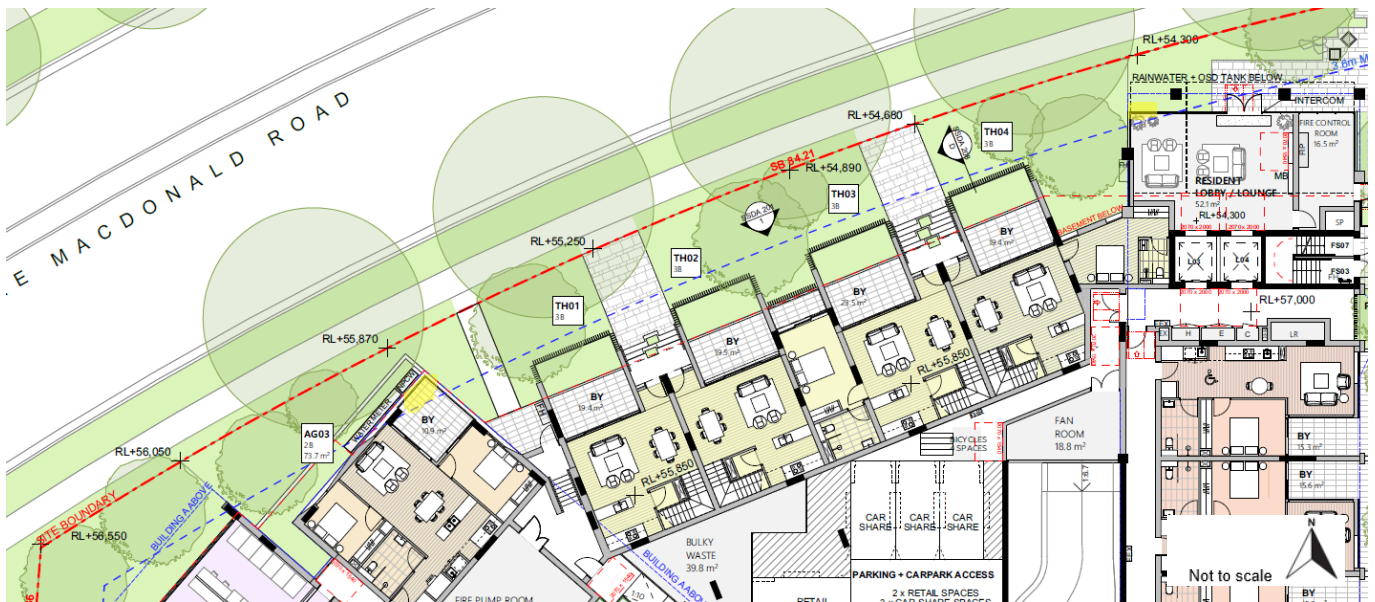
Figure 28 Proposed 15-storey building setbacks at Ground Floor level with encroachments to the 3.6m setback highlighted (source: FUSE, 2026)
