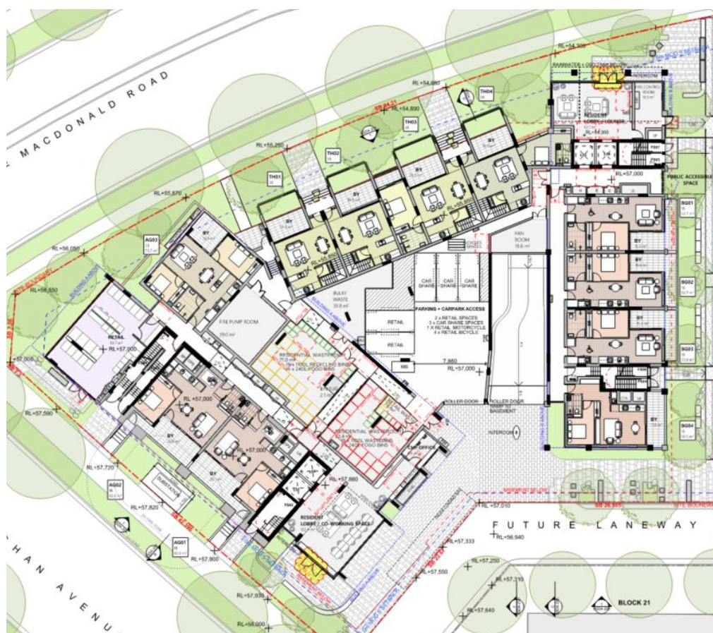
Figure 5 | Mark-up of the entrance doors required to be accessible |Source: Fuse Architects
