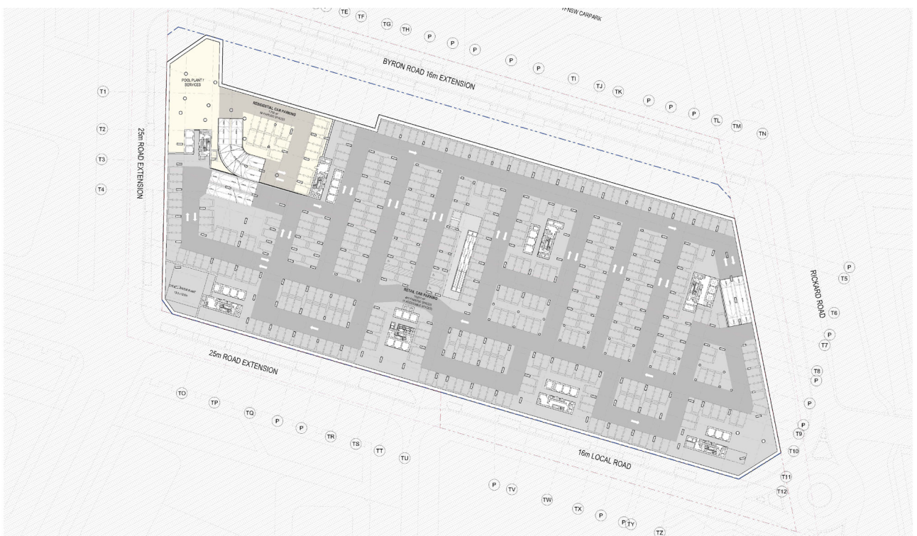
Figure 7 : Basement 2 - Retail Parking Level (DKO Architects 2025)
