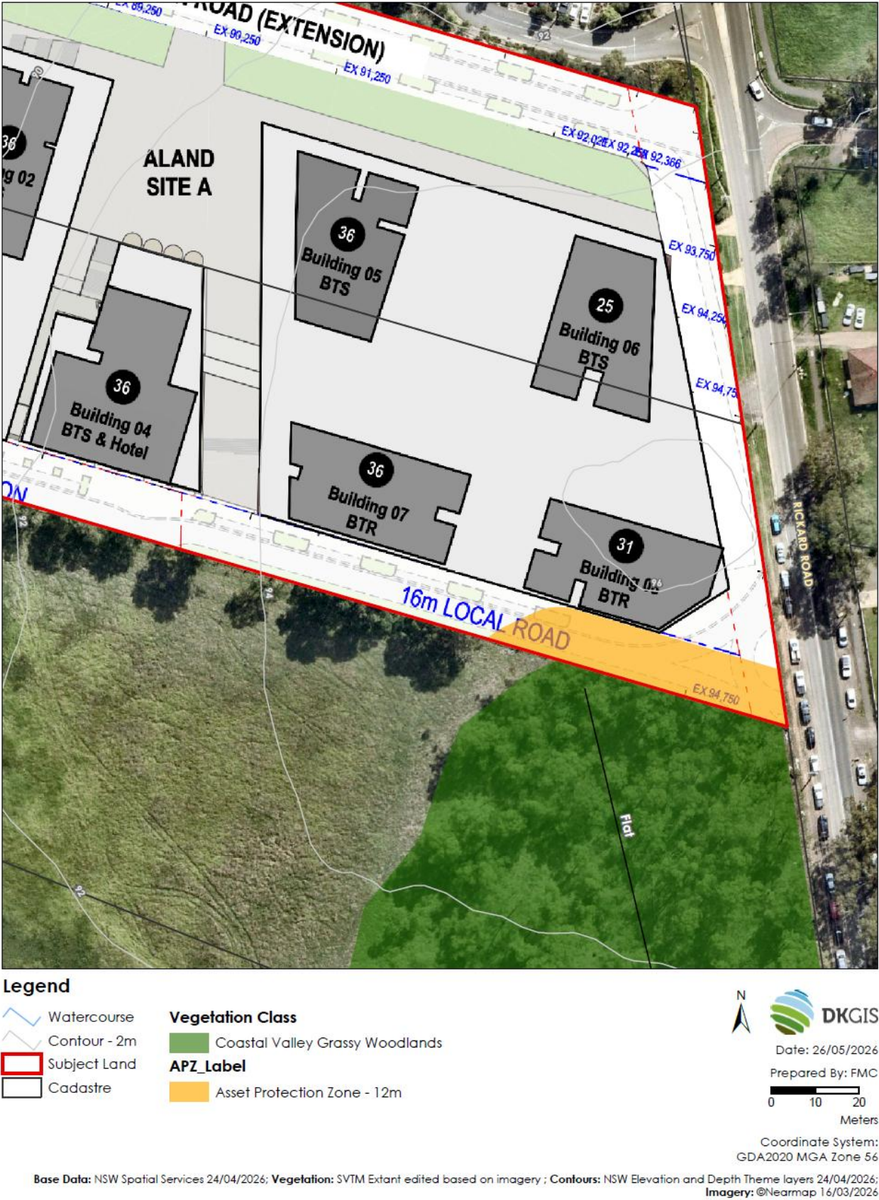
Figure 6: Minimum required Southeast APZ.
