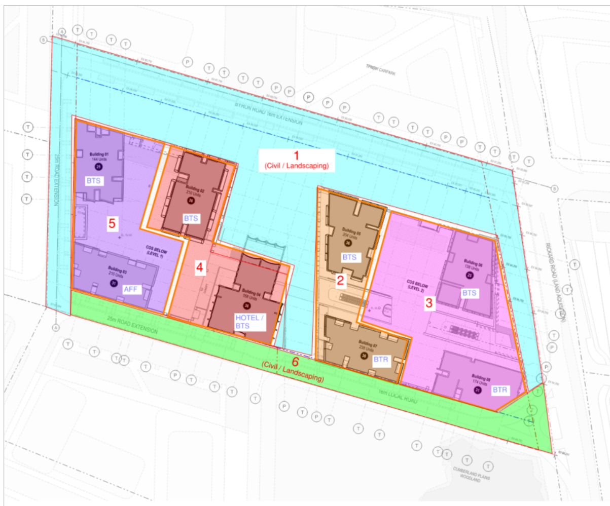
Figure 2: Reference Construction Staging Plan
