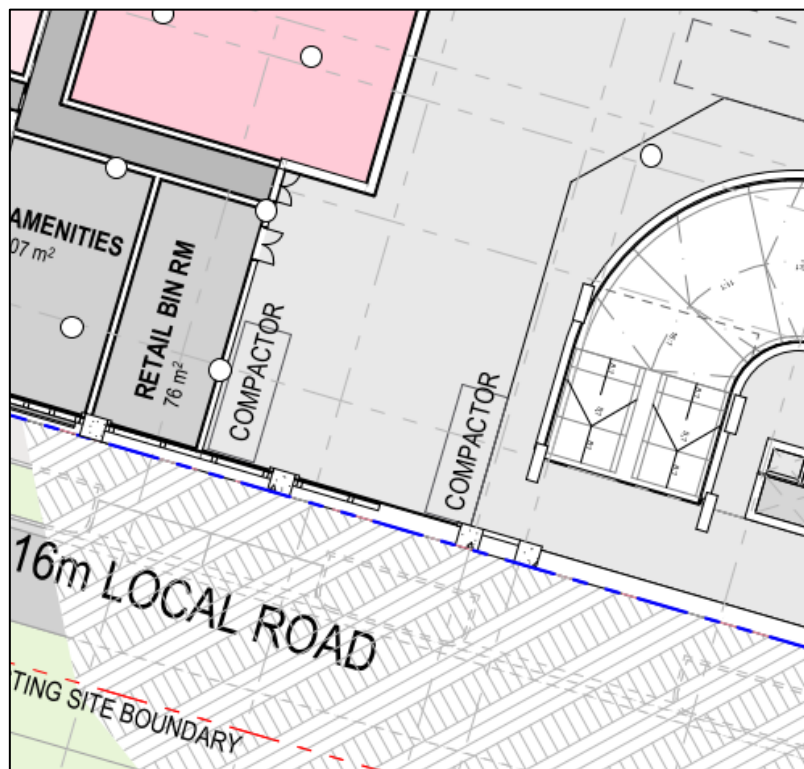
Figure 3 – Location of Compactor in Loading Dock
