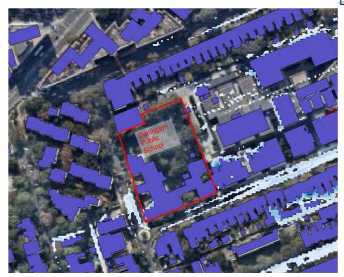
Figure 15 Flood Extent - 100 Year ARI (with 50mm Water Depth Cut-off)
