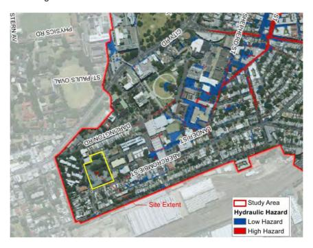
Figure 13 Flood Map – 100 Year ARI Design Flood Event (WBA Water dated September 2015)
