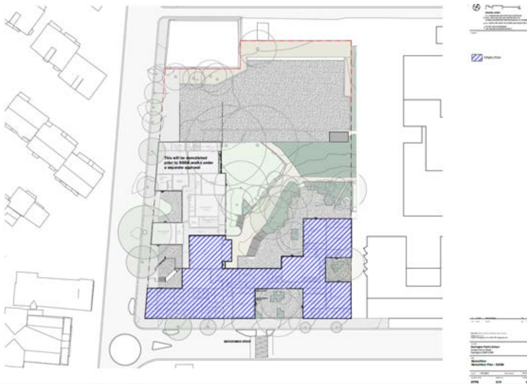
Figure 6.1 Demolition plan for Stage 2 demolition. Stage 1 demolition will be will take place under a separate authority. (Source: FJMT, April 2020) (refer also to figures 6-13 to 6-15 which show locations of retained and demolished murals).
