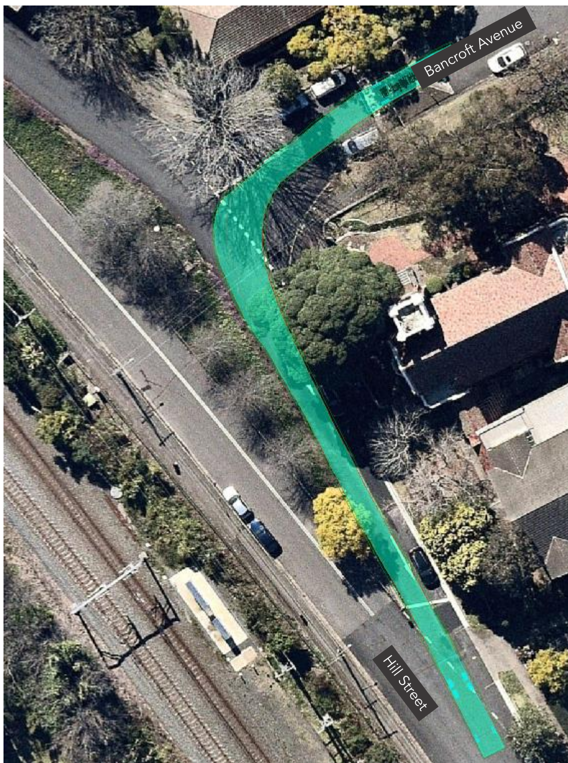
Figure 4.9 – Swept Path Analysis – HRV at intersection 6 (Hill Street/Bancroft Avenue)
