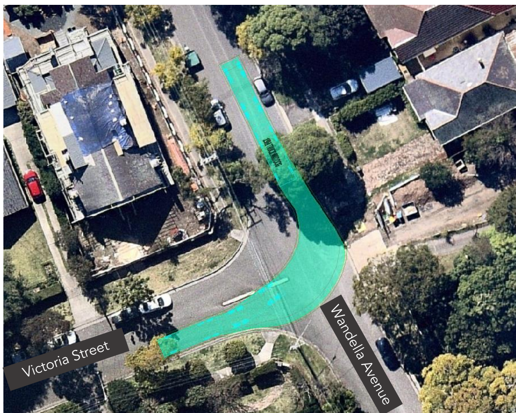
Figure 4.7 – Swept Path Analysis – 19m Truck and Dog at intersection 4 (Wandella Avenue/Victoria Street)
