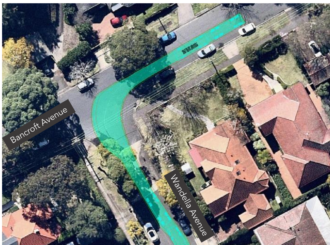
Figure 4.6 – Swept Path Analysis – 19m Truck and Dog at intersection 3 (Bancroft Avenue/Wandella Avenue)
