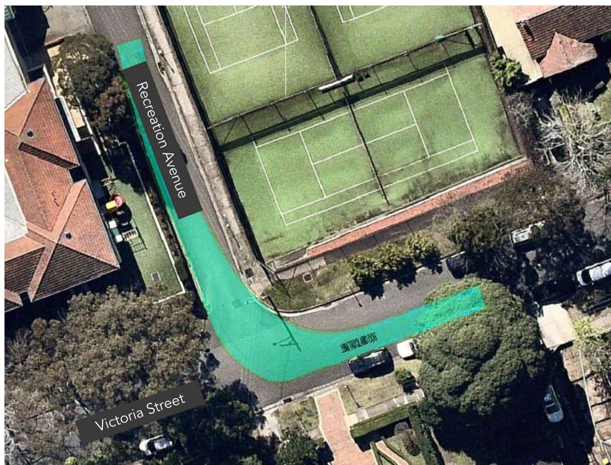
Figure 4.8 – Swept Path Analysis – 19m Truck and Dog at intersection 5 (Victoria Street/Recreation Avenue)
