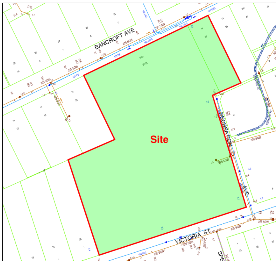
Figure 1 – Sydney Water - Sewer Mains
