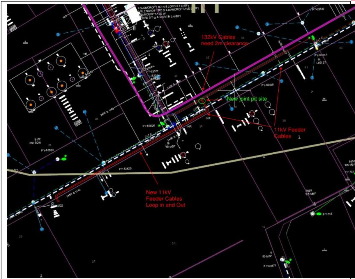
Figure: Existing 132kV and 11kV Underground cables and Proposed Loop in and Out arrangement
