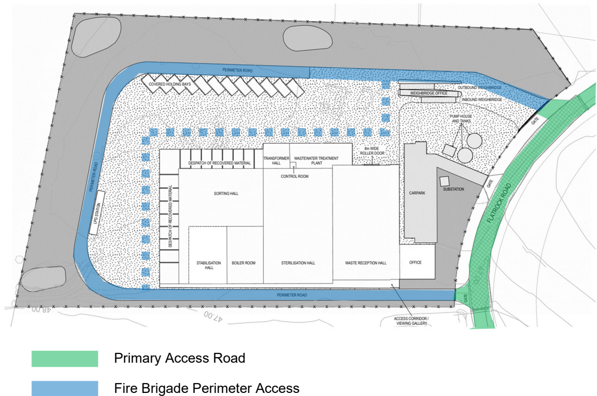
Figure 2.5 Indicative mark-up of access for FRNSW vehicles
