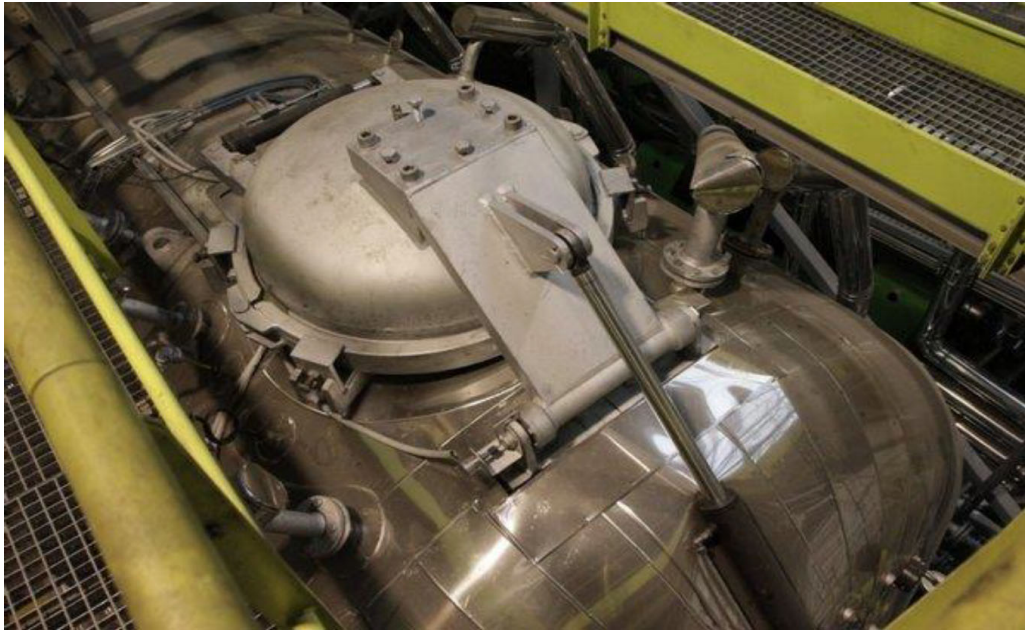
Photo 8.3 Autoclave jacket and waste loading hatch (example)
