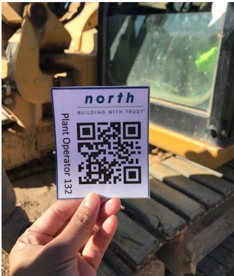
Photo 9 – QR code used for plant and equipment maintenance.
