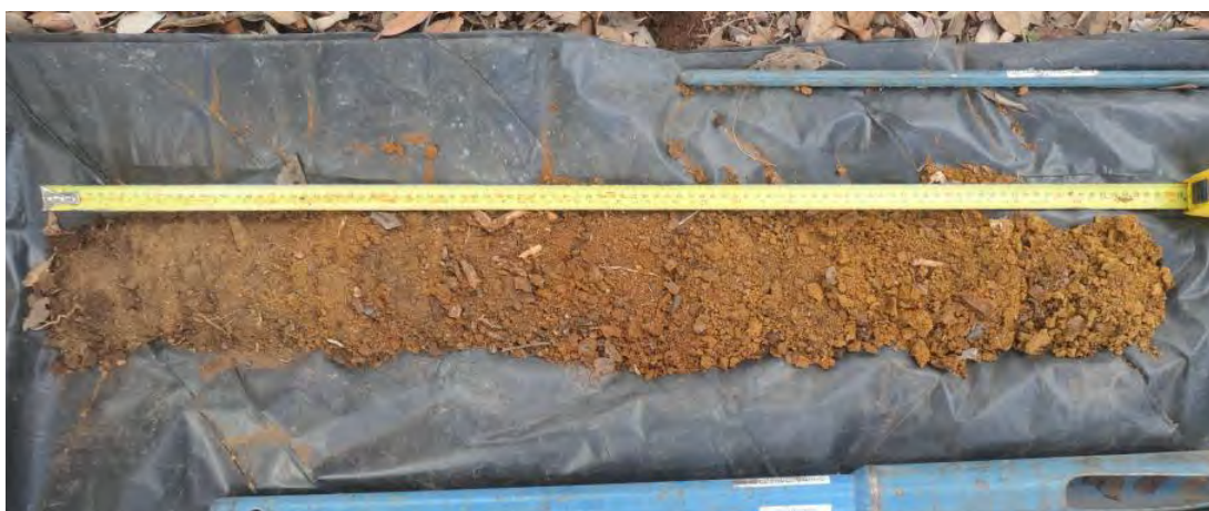
Figure 2.15 – Soil sample taken to a depth of 1.0m. (Photo: Arterra 1 November 2023)
