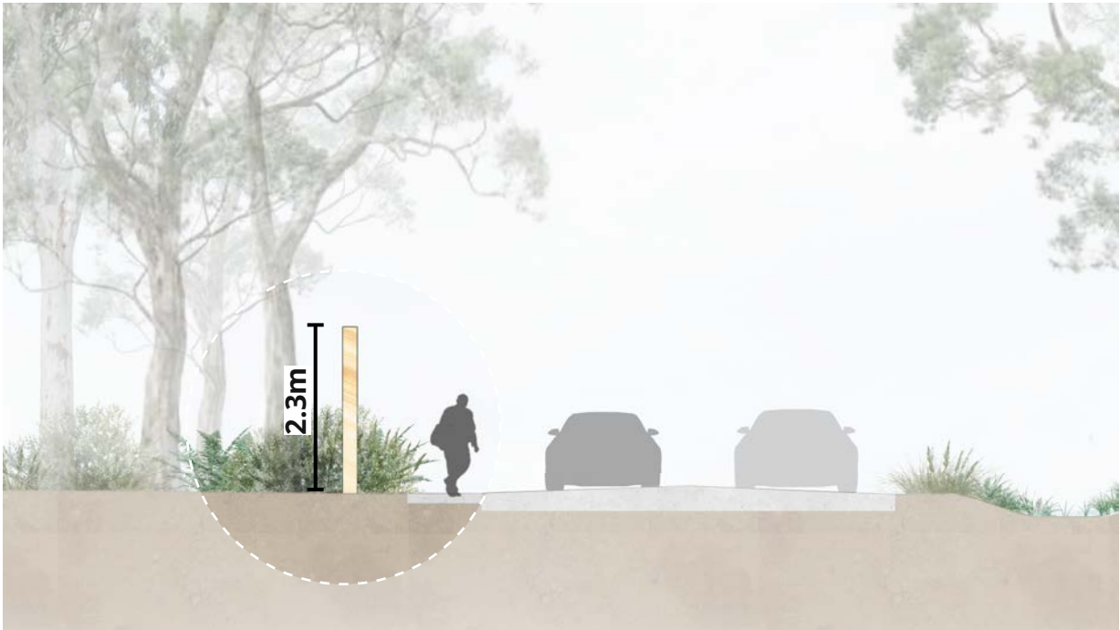
Fence Type A: HVM barrier fence
