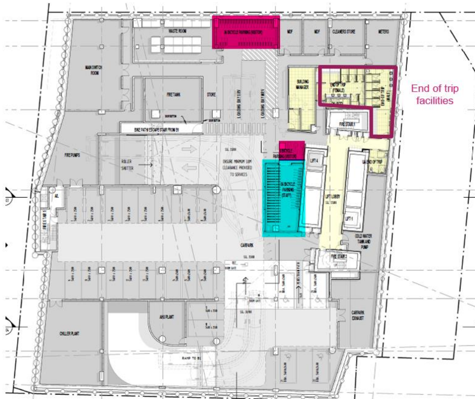
Figure 12: End-of-trip facilities within basement
