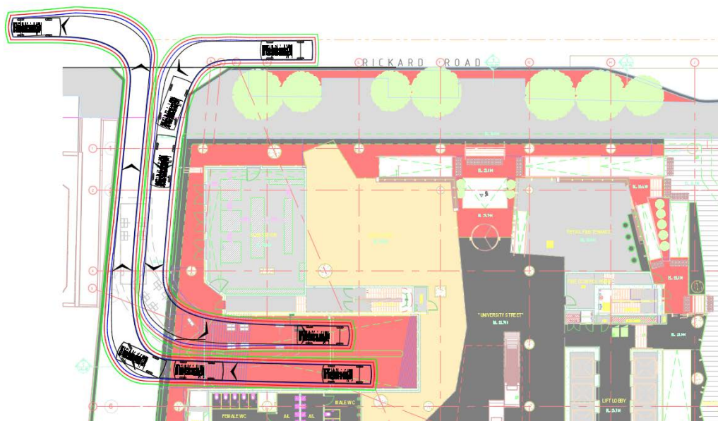
Figure 26 Access route to BCC basement car park
