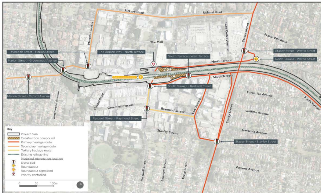
Figure 7 Metro construction routes
