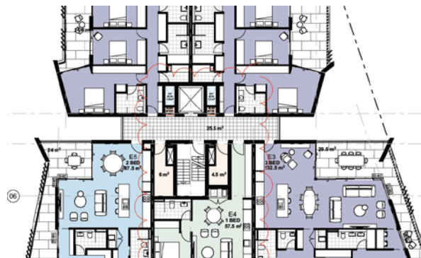
Figure 5 | Proposed Level 1-6 Plan with lift core, stairs, storerooms and internal layout of apartments changed
