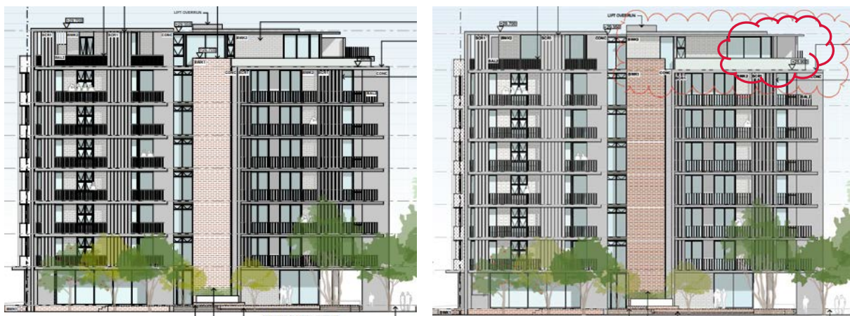
Figure 8 | East Elevations – approved on the left and proposed on the right – showing extension of typical Level 7 apartments to the north
