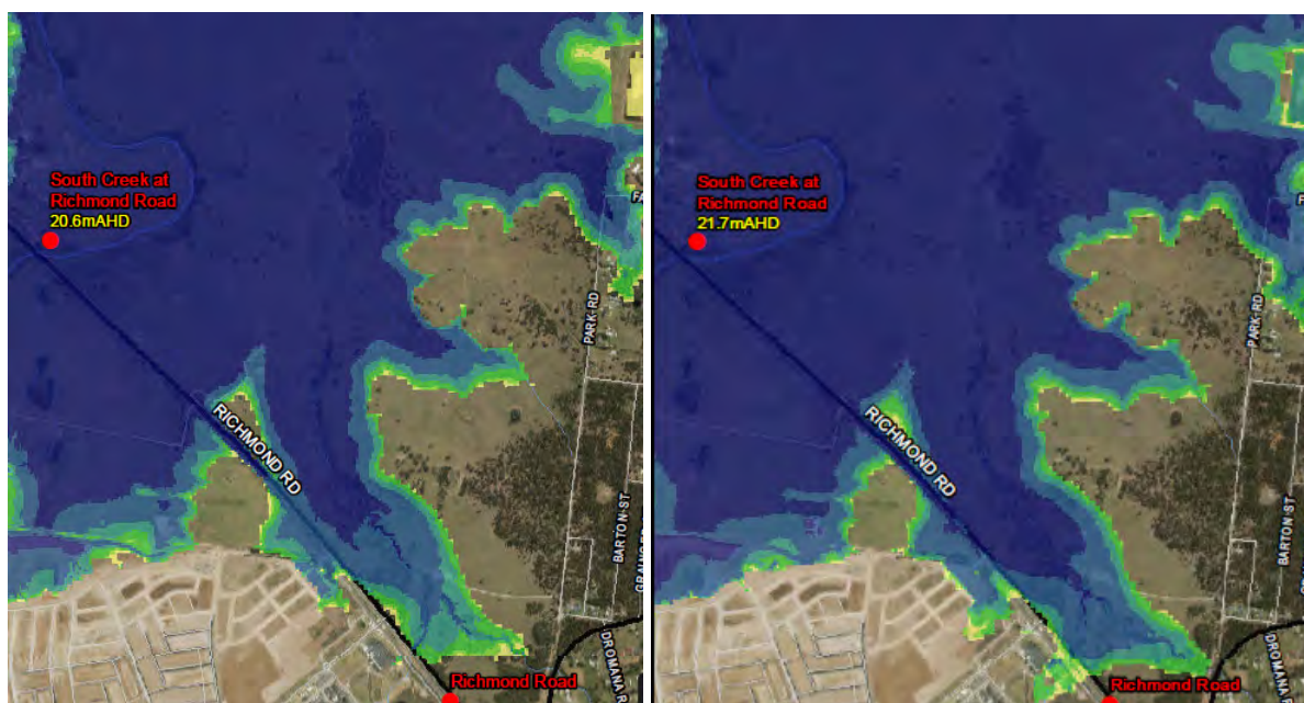
Figure 10 & 11: 0.1% AEP Flood extent and Level (left), 0.05% AEP Flood Extent and Level (right), HNVRFs2019.
