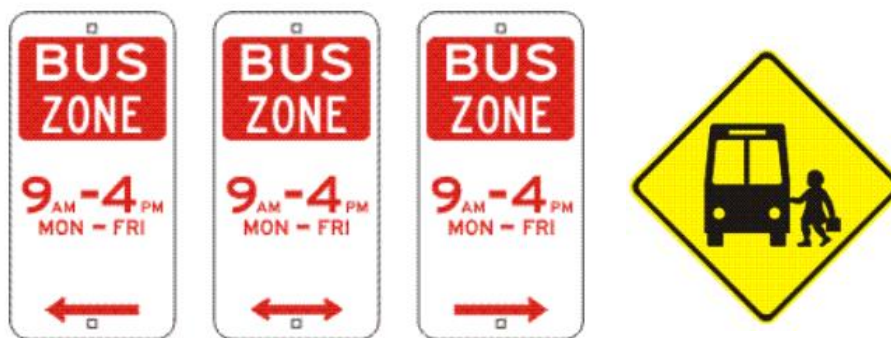
Figure 3-6 – Examples of Bus Zone Signage
