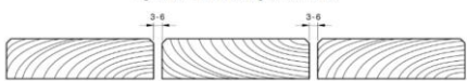
(a) Gap spacing for continuous timber and composite decking * Gaps may be increased to 10 mm in high rainfall areas for exposed installations and boards exceeding 150 mm width
