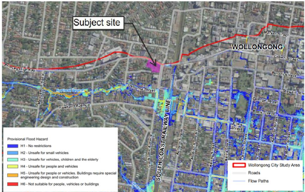
Figure 8 Flood Hazard risk for site
