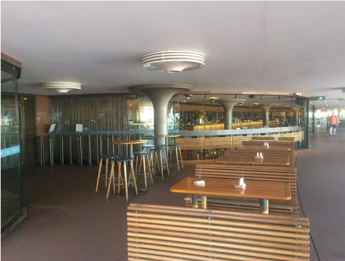
Figure 7: Lower Concourse mushroom columns and louvered disc light fittings (Source: Keylan)
