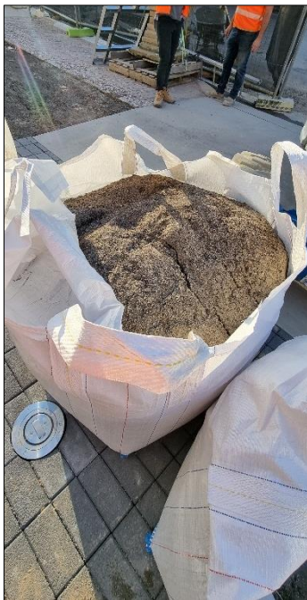
Figure 32 – Packing sand from Saddingtons used for Paving (28 July 2021 – supplied by Built).
