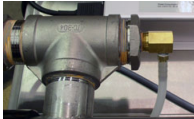
Installation on the Out Port with a T-Fitting
