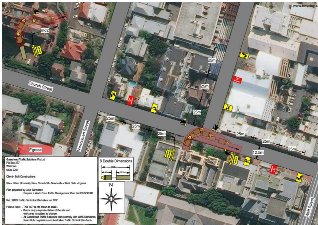
Figure 15: Building A vehicle egress from site to Church Street under traffic control
