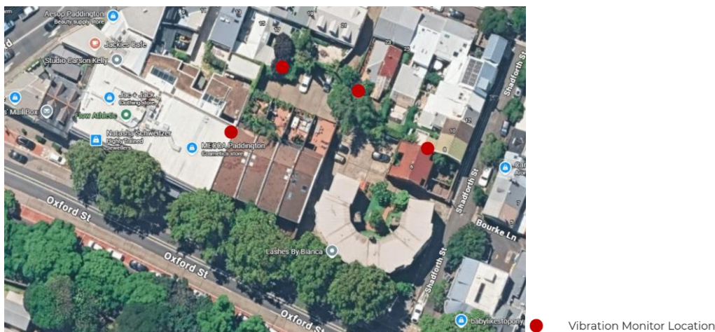
Figure 21 Location of Vibration Monitoring Points
