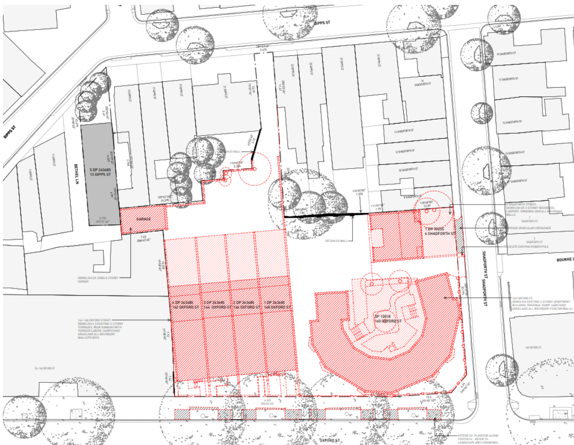
Figure 20 Demolition plan (demolished structures hatched outline)
