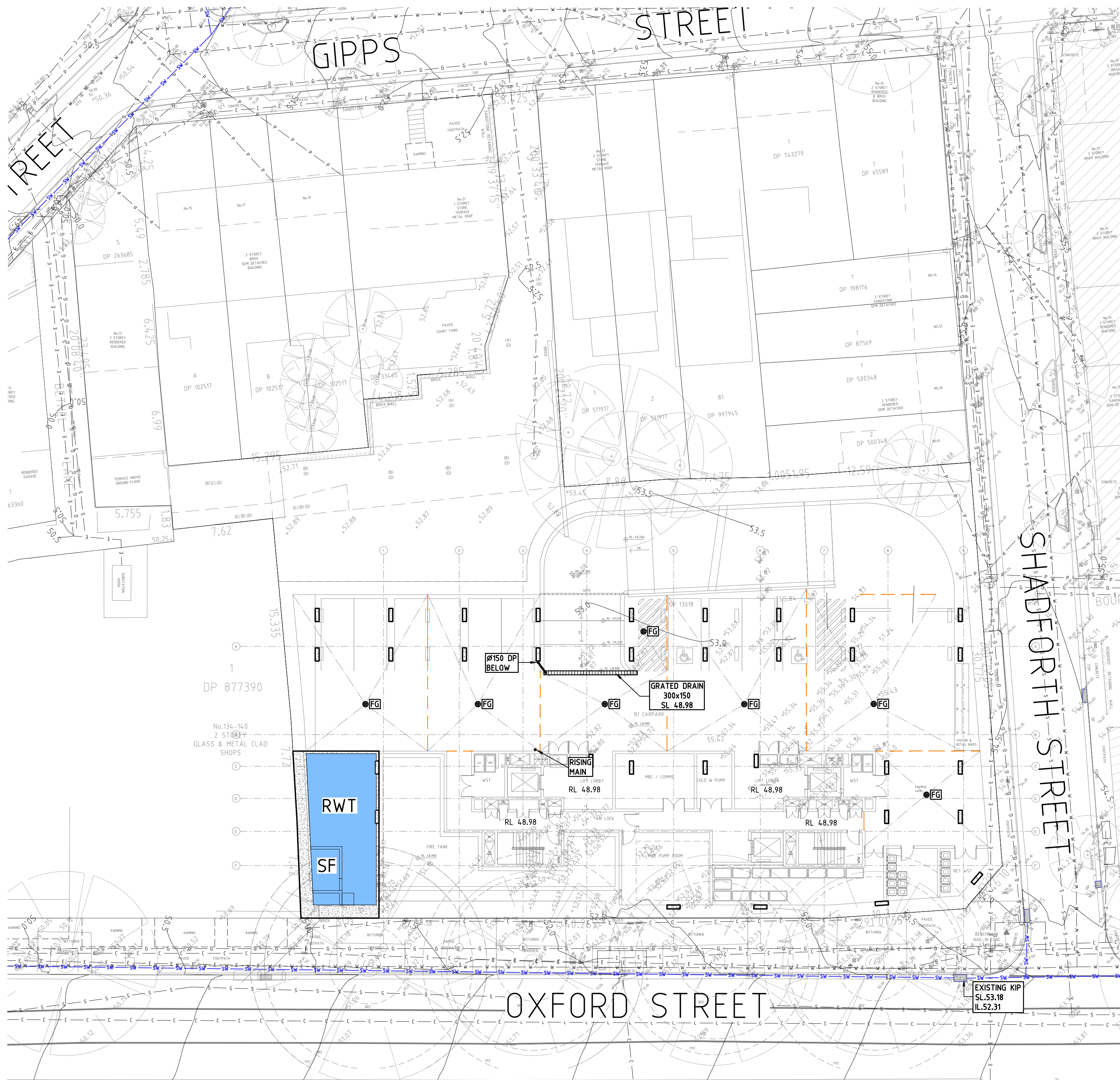
STORMWATER LAYOUT PLAN BASEMENT 1 LEVEL SCALE 1:200
