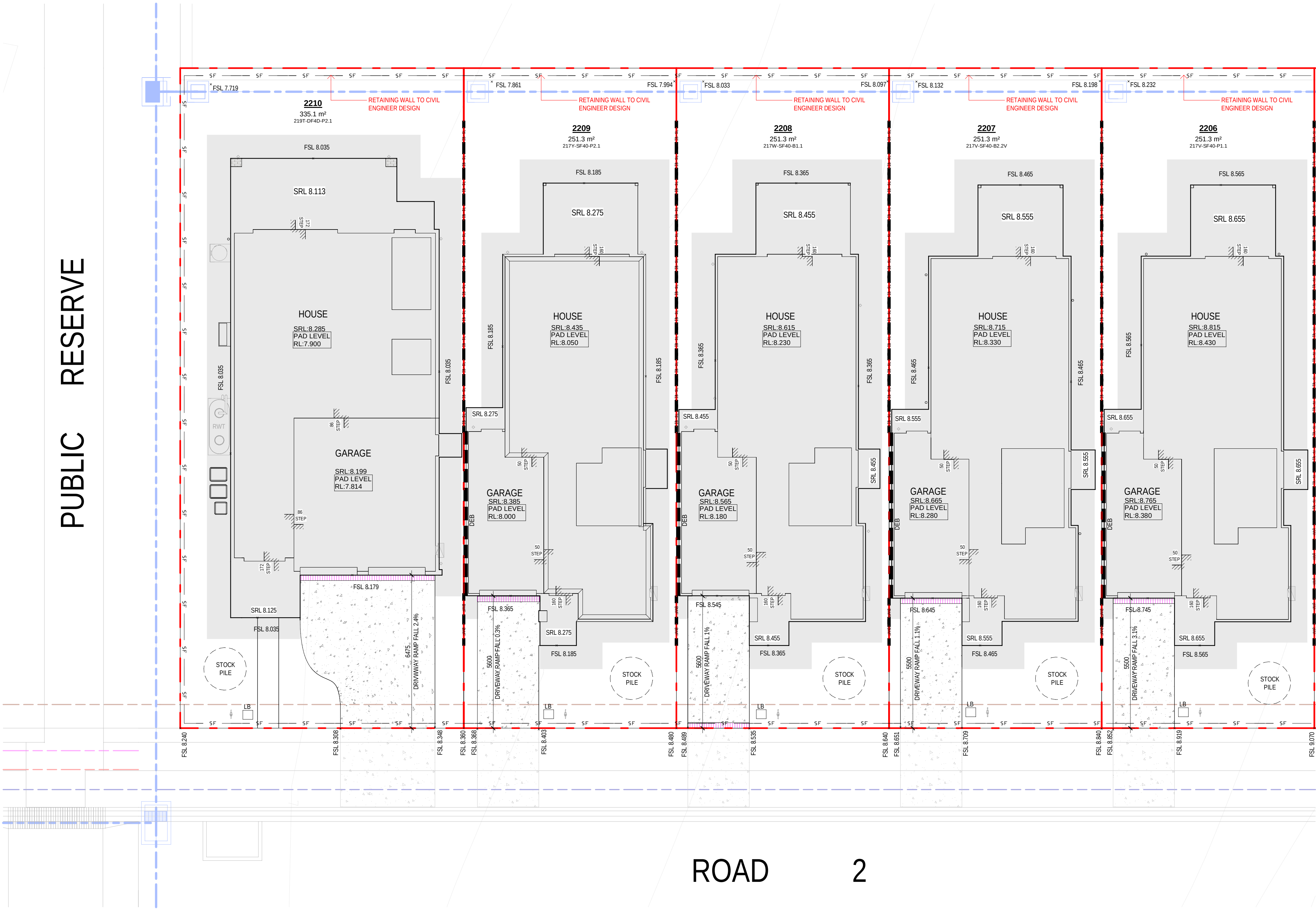
1 EROSION/SEDIMENT CONTROL & BENCHING PLAN - LOT 2206-2210 1 : 100
