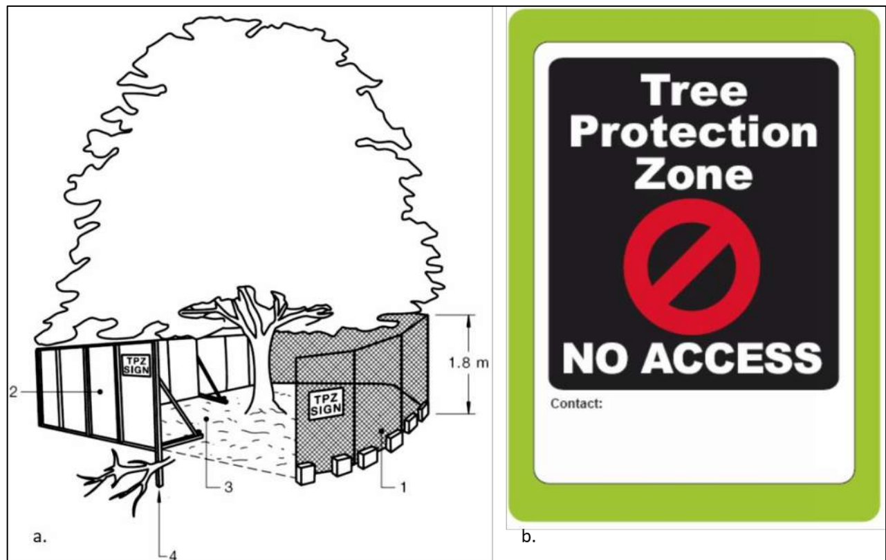
Figure 8. Protection fencing should be erected around the specified perimeter of TPZs in accordance with Section 4.3 of AS4970 (2009) . Figure 11 a. depicts correctly installed steel or plywood fence panelling (1 and 2) with mulch inside the protection area (3). Figure 11 b. shows depicts protection fencing signage.
