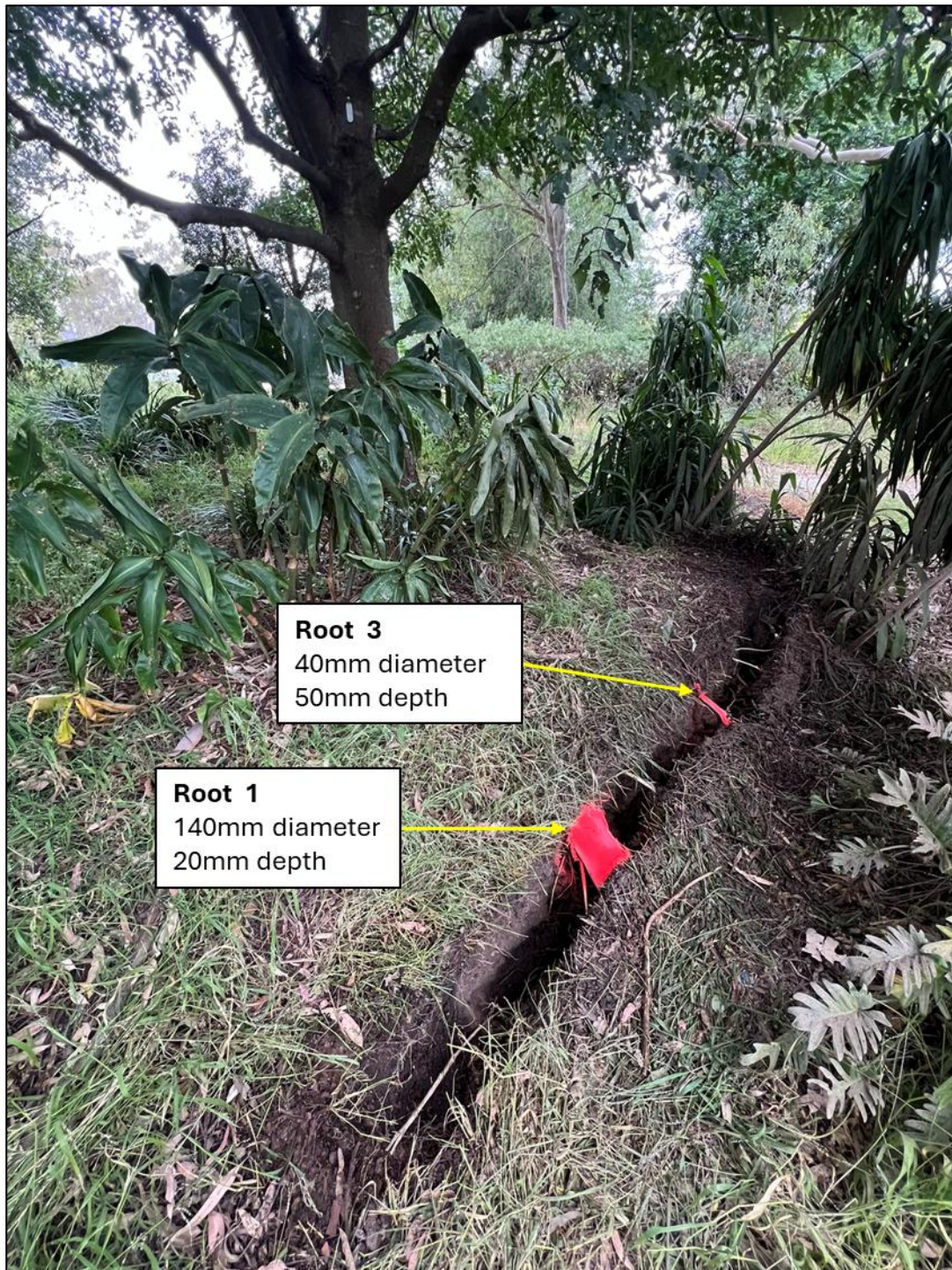
Figure 64. Roots 1-3 in central portion of Survey Trench 17.
