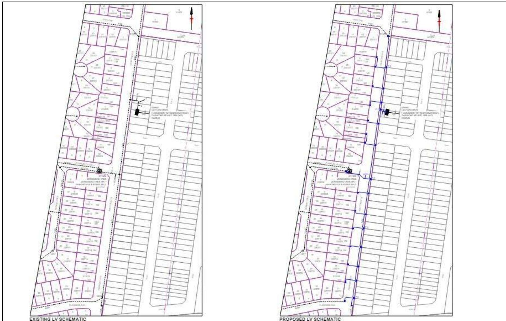
Figure 6: Underground Residential Subdivision-Stage 1: 271 Horsely Road, Milperra, NSW , prepared by Edgewater Connections (Ausgrid Project No: AN-25851, Sheet 6 of 7. Annotated by Temporal Tree Management Pty Ltd. (17/05/2024). Proposed underground LV electrical service locations are annotated in BLUE.
