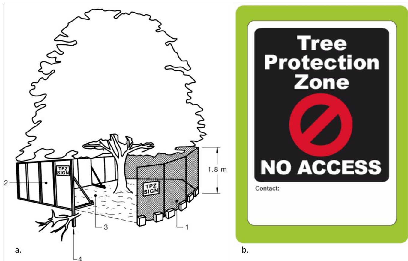
Figure 8. Protection fencing should be erected around the specified perimeter of NRZs in accordance with Section 4.3 of AS4970 (2025) . Figure 8 a. depicts correctly installed steel or plywood fence panelling (1 and 2) with mulch inside the protection area (3). 8 b. shows protection fencing signage.
