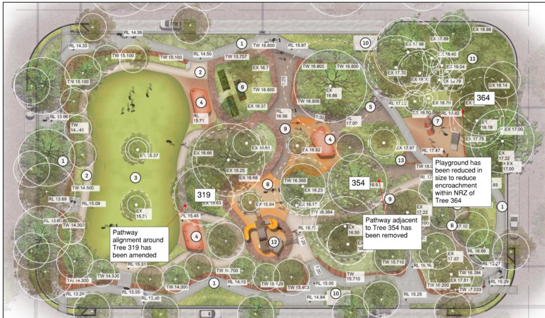
Figure 9. Updated Landscape Concept Plan for Central Park with incorporated design amendments based on findings from the Root Mapping Assessment undertaken between 20-28/10/2025.
