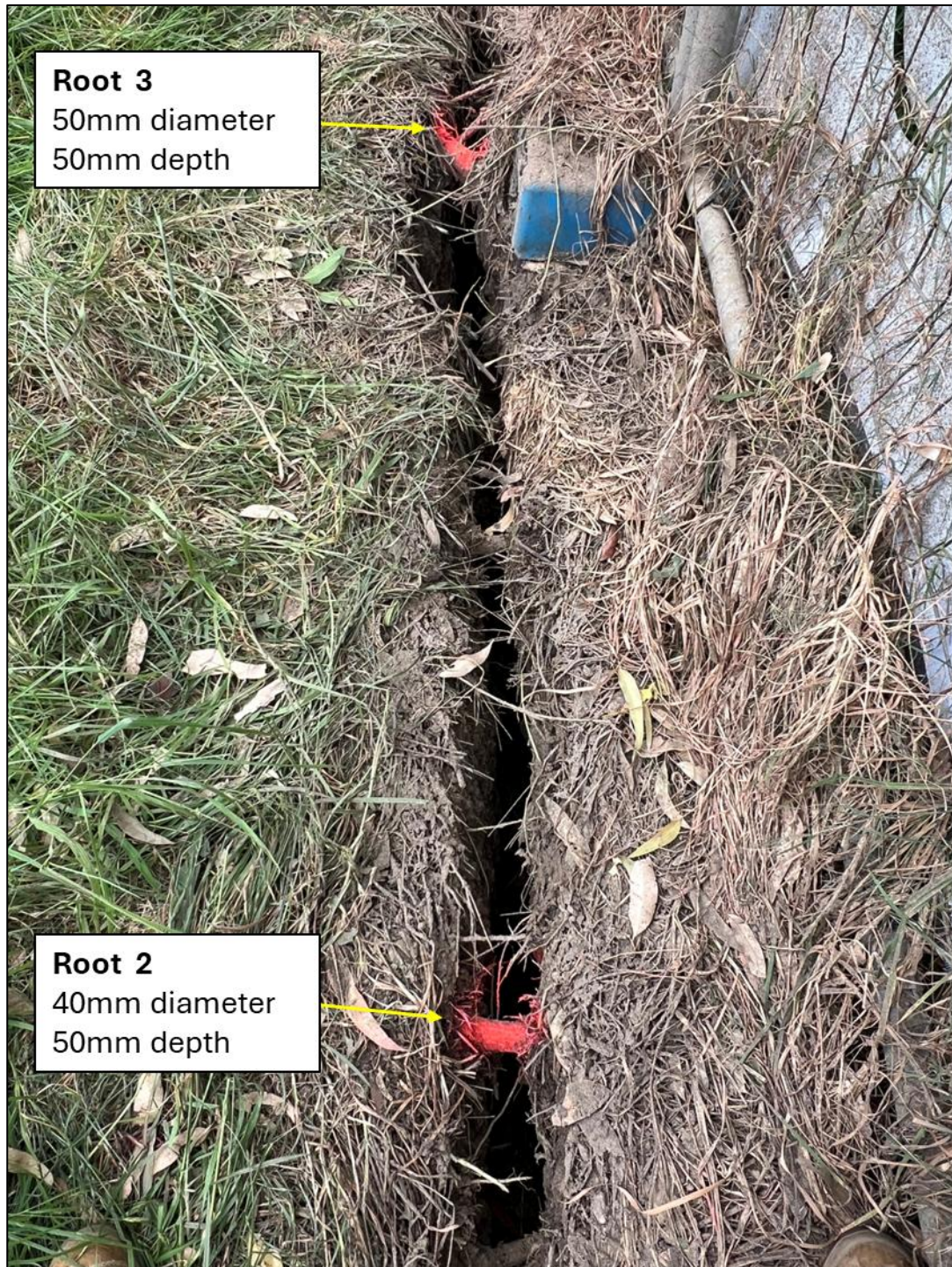
Figure 39. Roots 2 and 3 within central portion of Survey Trench 10.
