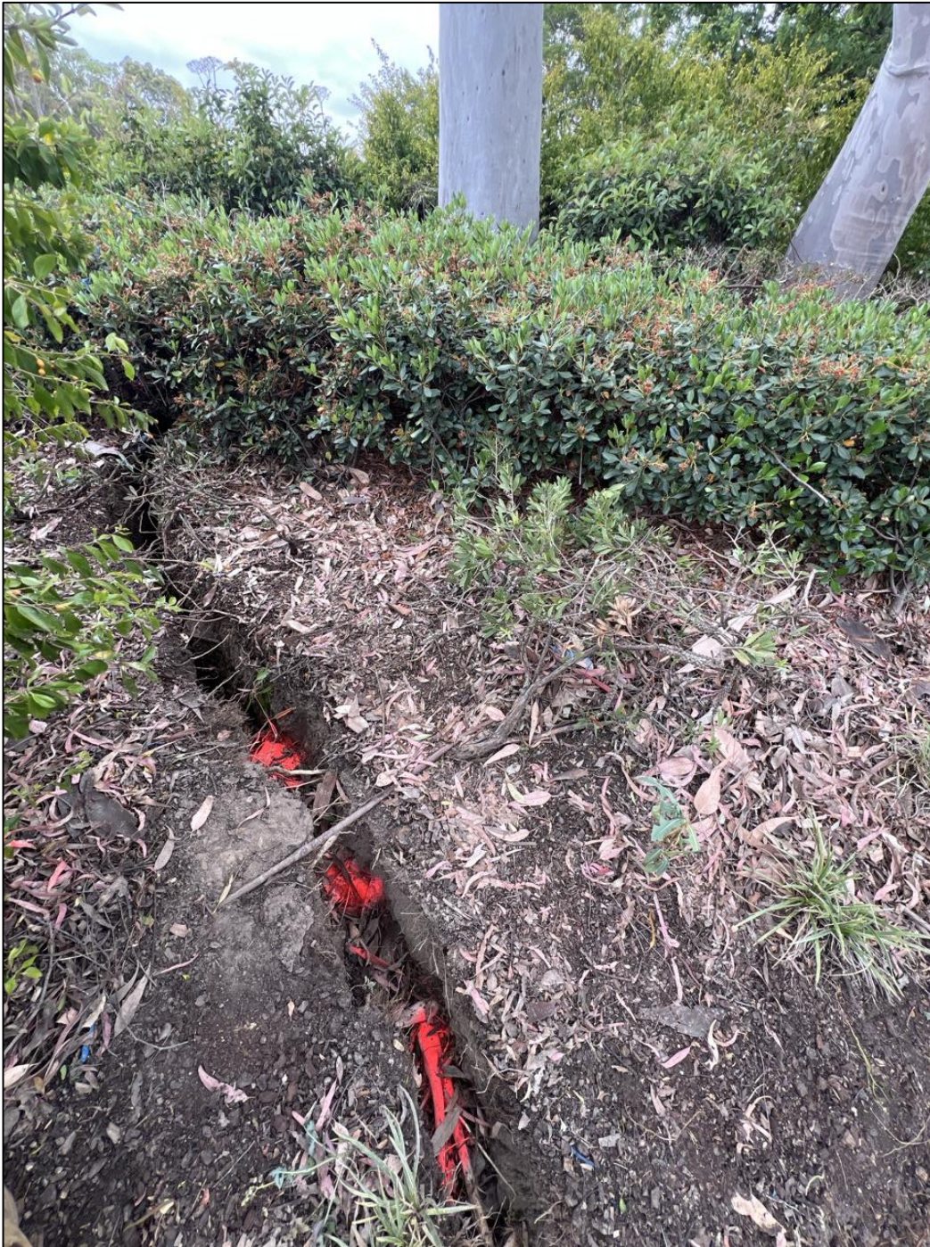
Figure 50. Trench 13 with three major roots encountered. Image taken from south-eastern edge of trench.
