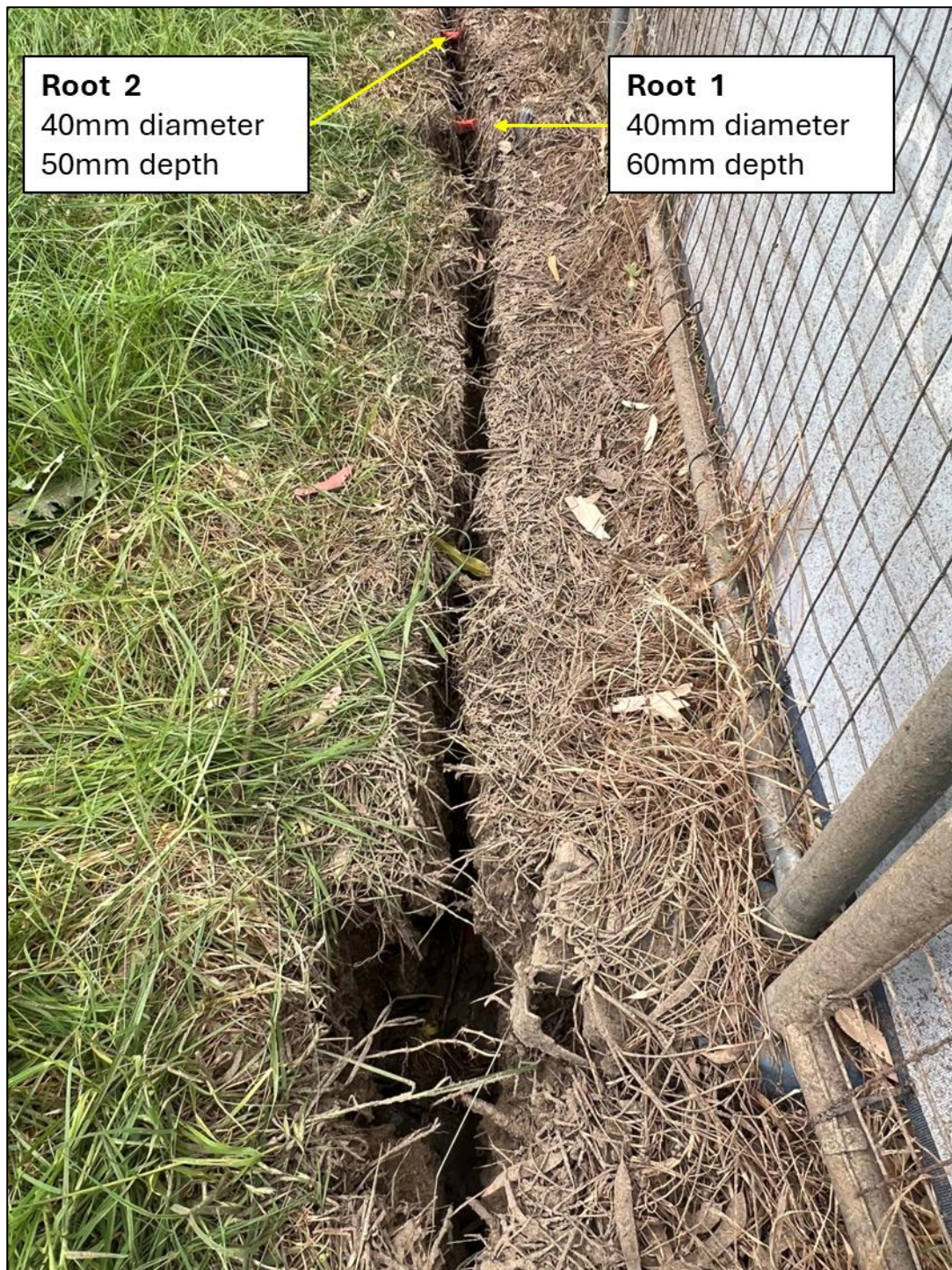
Figure 37. Roots 1 and 2 within central portion of Survey Trench 10. No major roots observed within eastern portion of trench.
