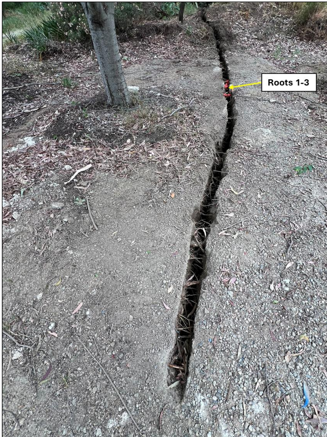
Figure 55. Roots 1-3 in western portion of Survey Trench 14 adjacent to Tree 341.
