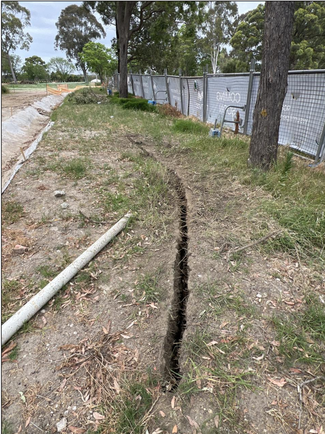
Figure 29. Trench 6 with no major or minor roots encountered. Image taken from northern edge of trench.
