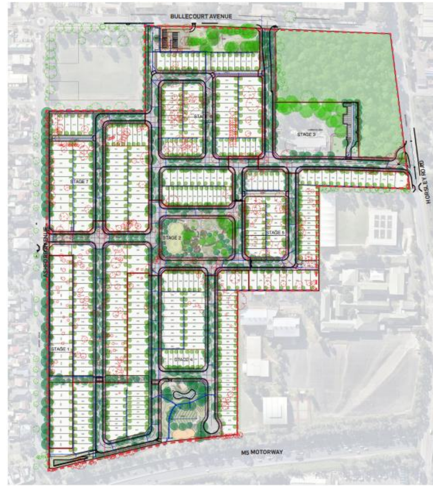
Figure 7. Proposed tree replacement strategy and canopy coverage percentages within the site prior to and after required tree clearing and after tree replanting.
