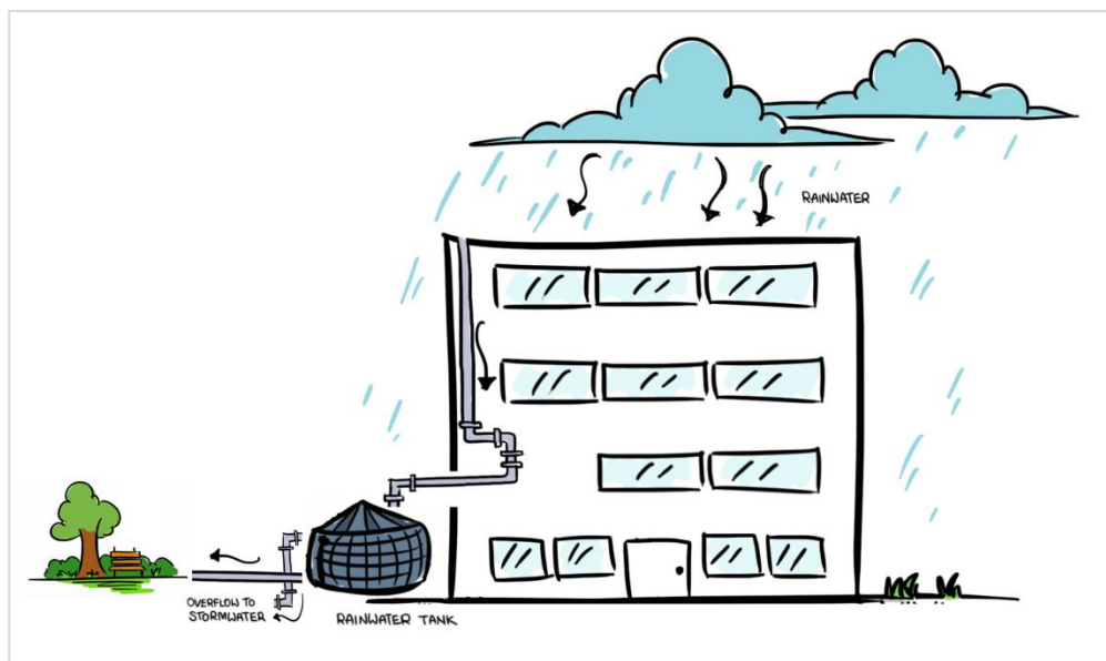
Figure 6: Rainwater harvesting system for landscape irrigation
