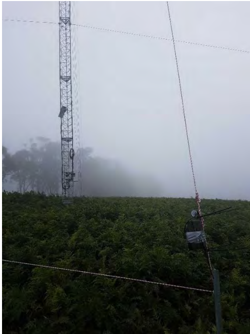
Photo 8 Met mast deployed acoustic detector at head height
