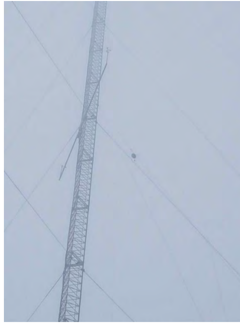
Photo 9 Met mast deployed acoustic detector at aerial height
