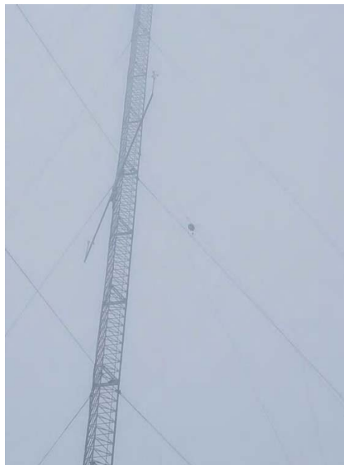
Photo 9 Met mast deployed acoustic detector at canopy height
